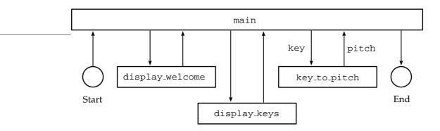
Each of the structural units in the diagram is a function. These functions are documented in the table below:
