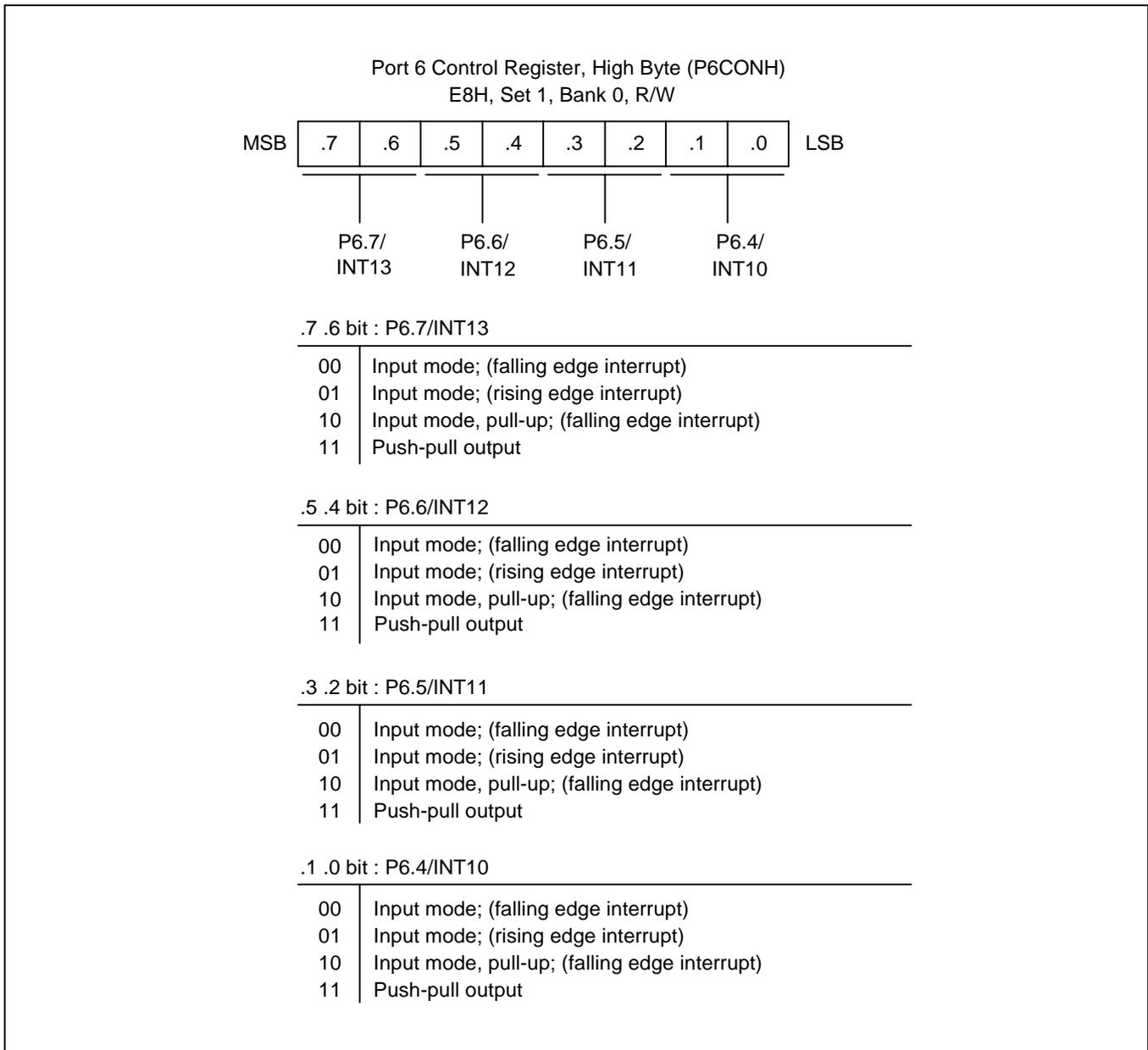
**Figure 9-14. Port 6 High-Byte Control Register (P6CONH)**
