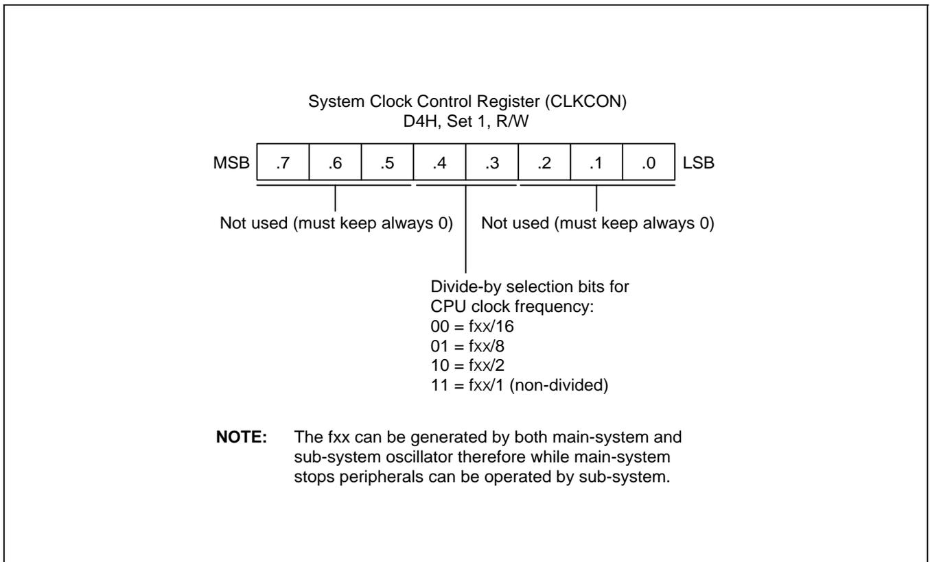
**Figure 7-4. System Clock Control Register (CLKCON)**
