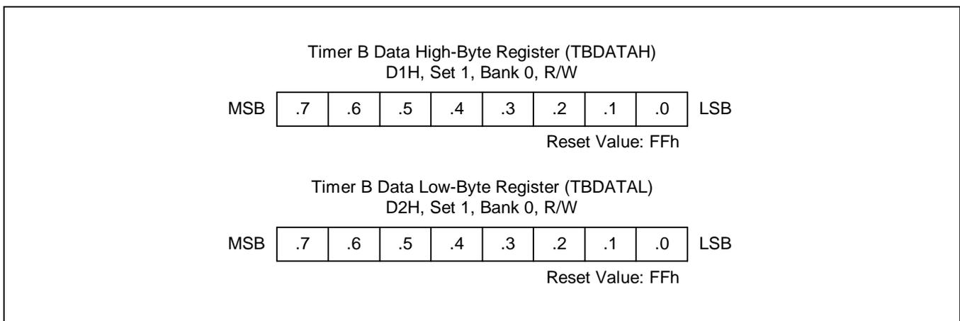
Figure 11-5. Timer B Data Registers (TBDATAH, TBDATAL)
