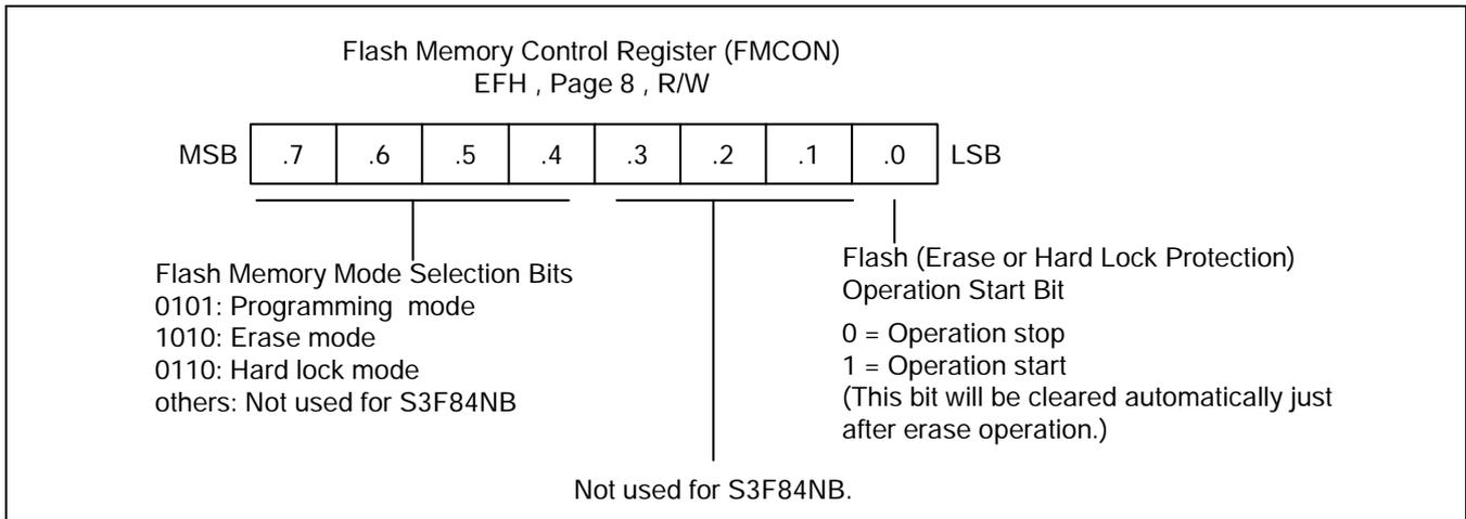
**Figure 19-3. Flash Memory Control Register (FMCON)**
