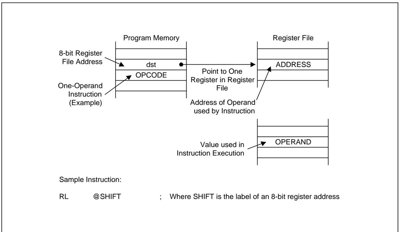
Figure 3-3. Indirect Register Addressing to Register File
