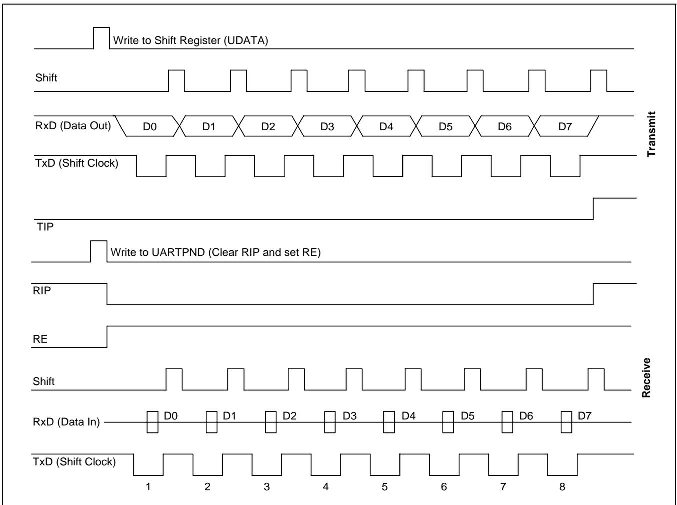
Figure 14-6. Timing Diagram for UART Mode 0 Operation
