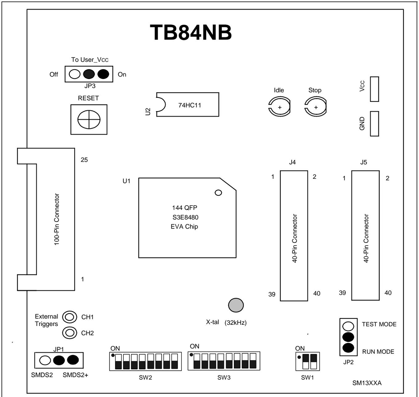
**Figure 22-2. S3F84NB Target Board Configuration**
