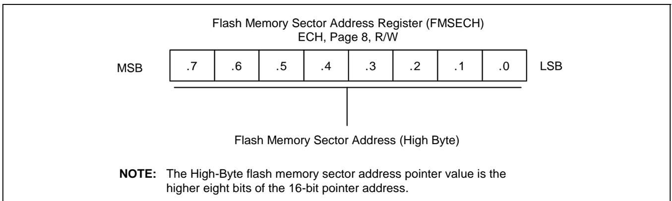
**Figure 19-5. Flash Memory Sector Address Register (FMSECH)**
