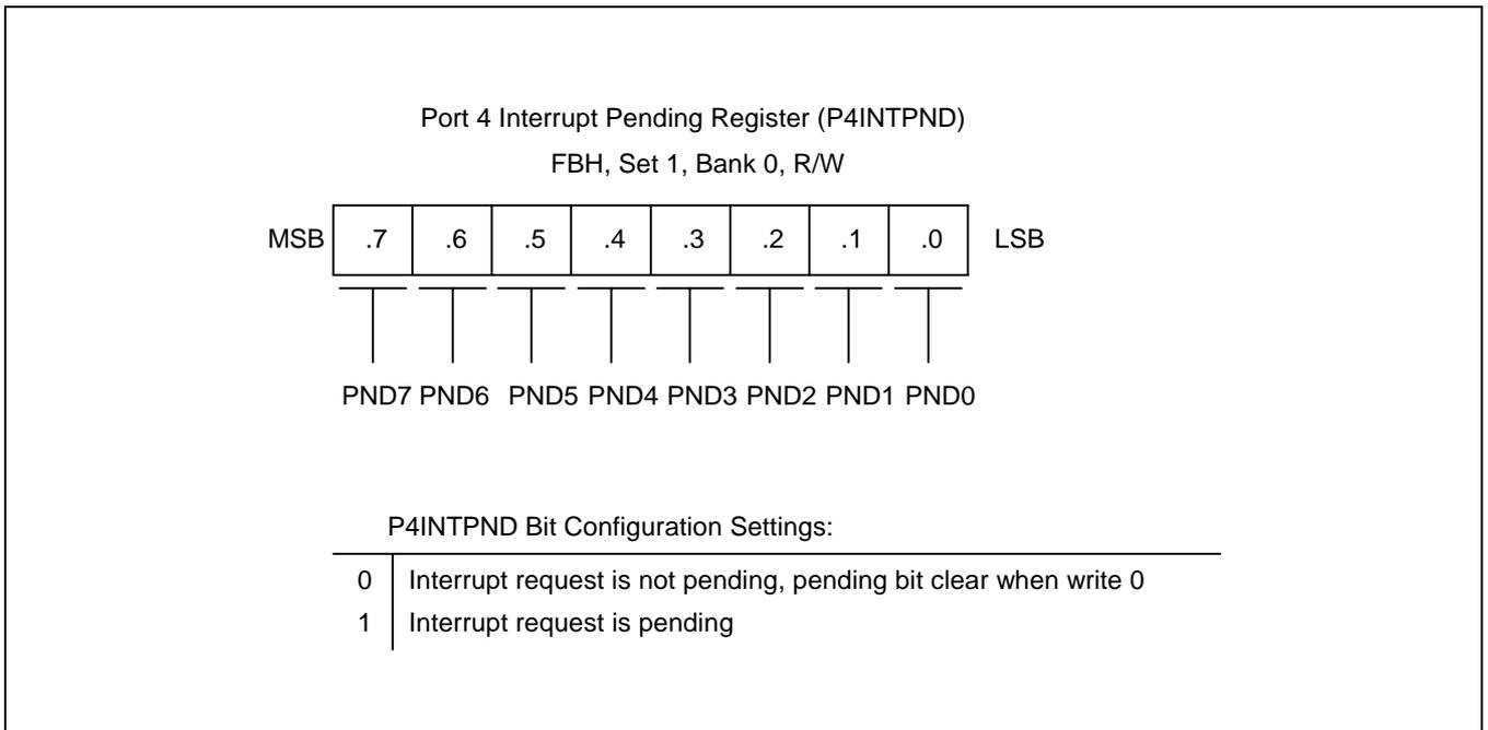
**Figure 9-11. Port 4 Interrupt Pending Register (P4INTPND)**
