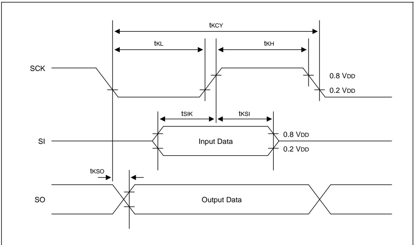
**Figure 20-8. Serial Data Transfer Timing**
