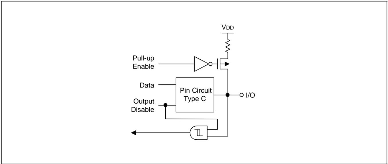
Figure 1-6. Pin Circuit Type D (Port 0, 2, 3 and P5.0-P5.3)
