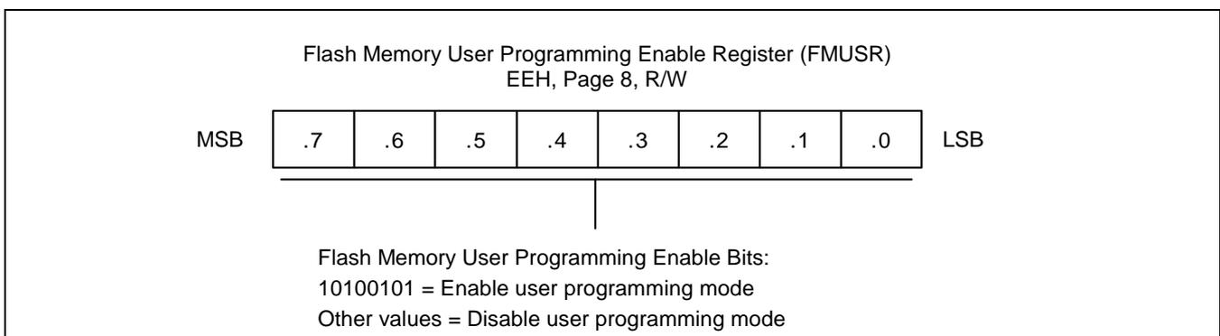
**Figure 19-4. Flash Memory User Programming Enable Register (FMUSR)**
