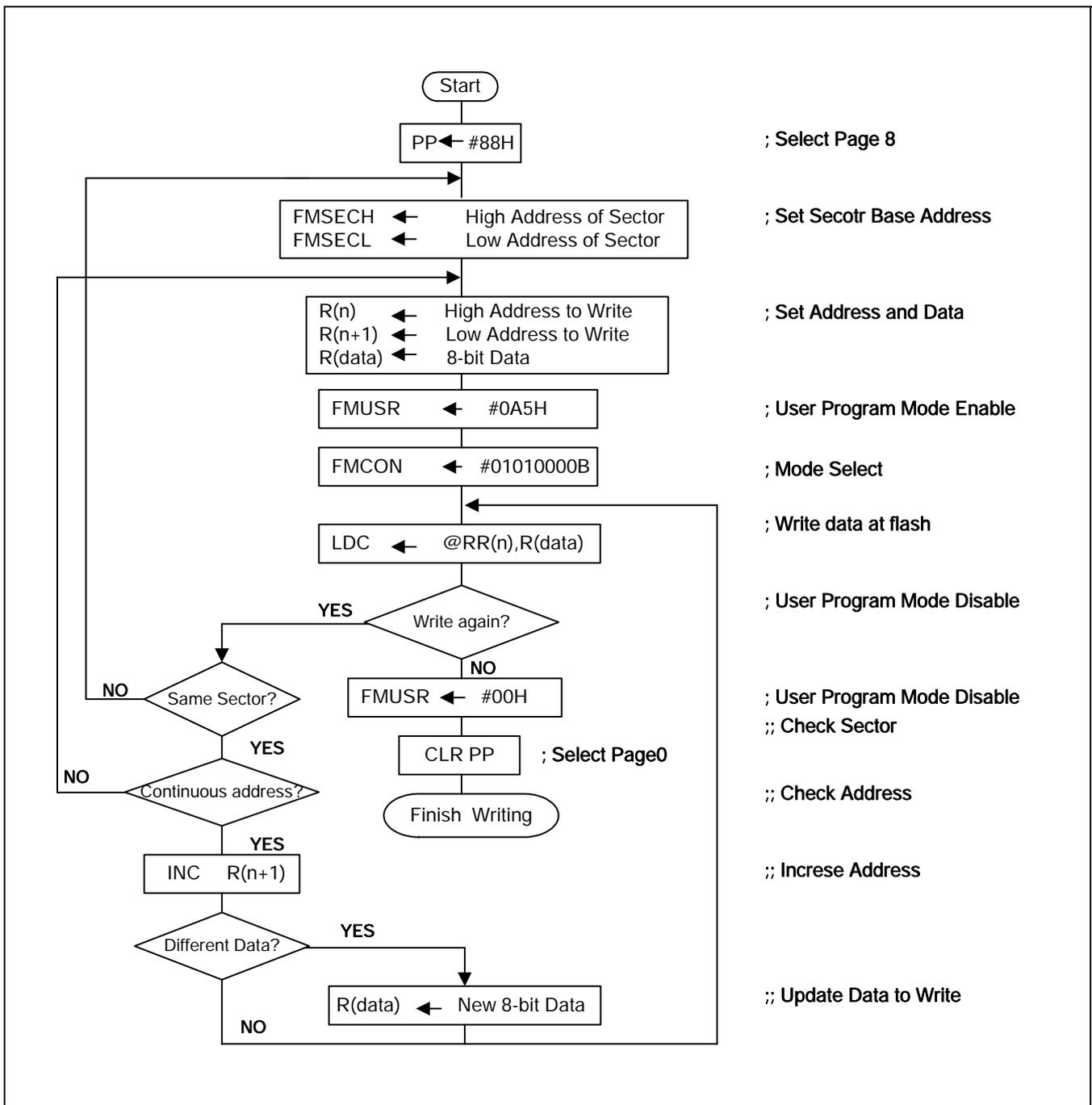
Figure 19-10. Program Flowchart in a User Program Mode
