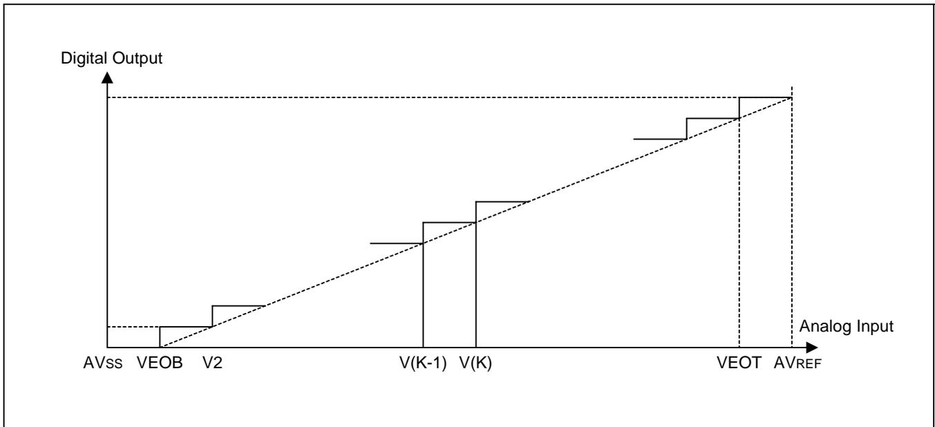
Figure 20-10. Definition of DLE and ILE
