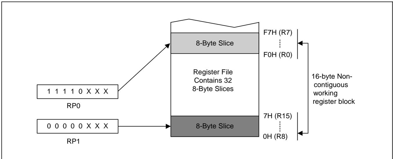
**Figure 2-8. Non-Contiguous 16-Byte Working Register Block**
