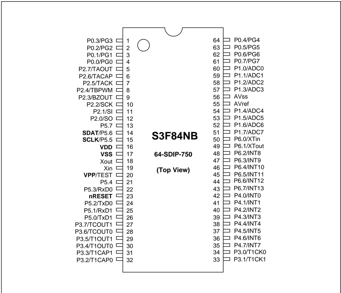
Figure 1-2. S3F84NB Pin Assignment (64-pin SDIP)
