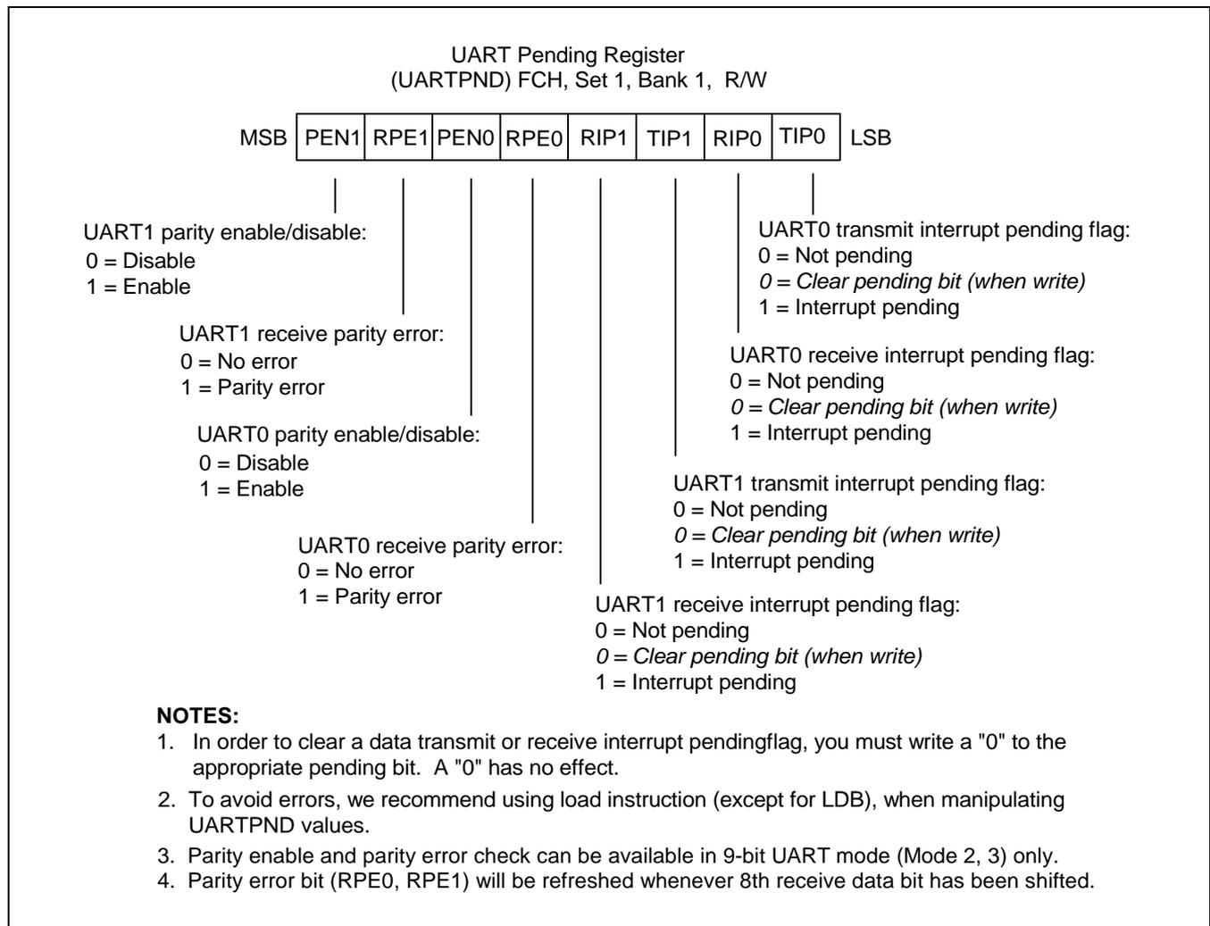
**Figure 14-2. UART Interrupt Pending Register (UARTPND)**
