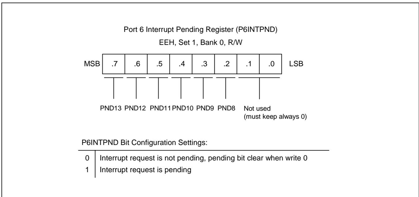
**Figure 9-17. Port 6 Interrupt Pending Register (P6INTPND)**
