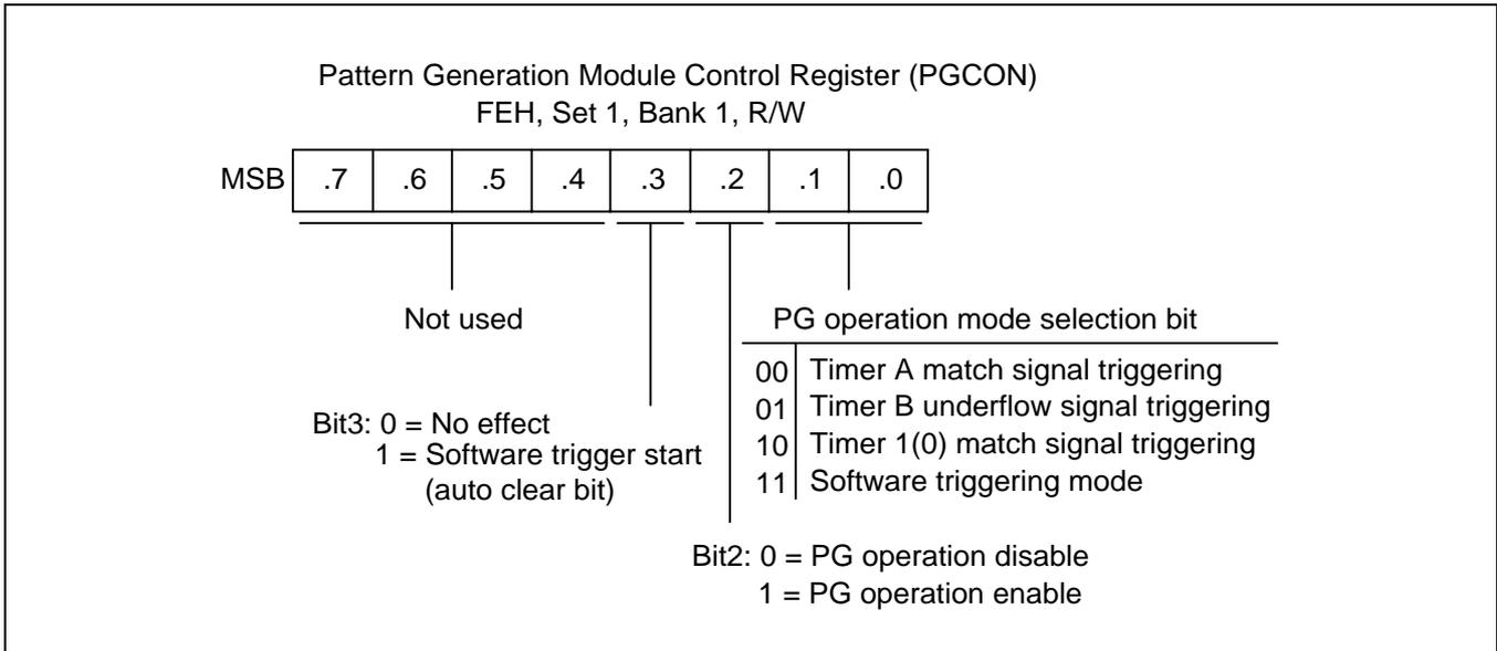
Figure 17-2. PG Control Register (PGCON)
