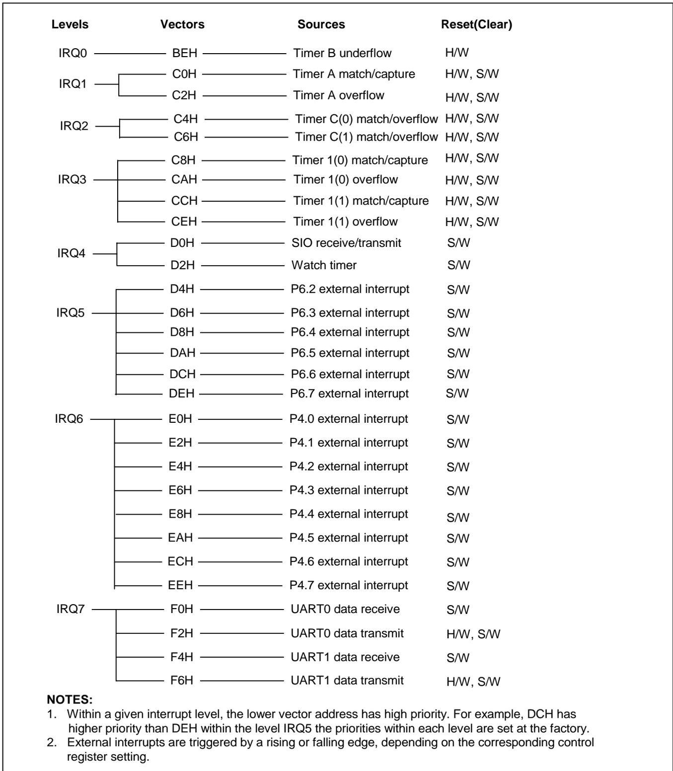
Figure 5-2. S3F84NB Interrupt Structure
