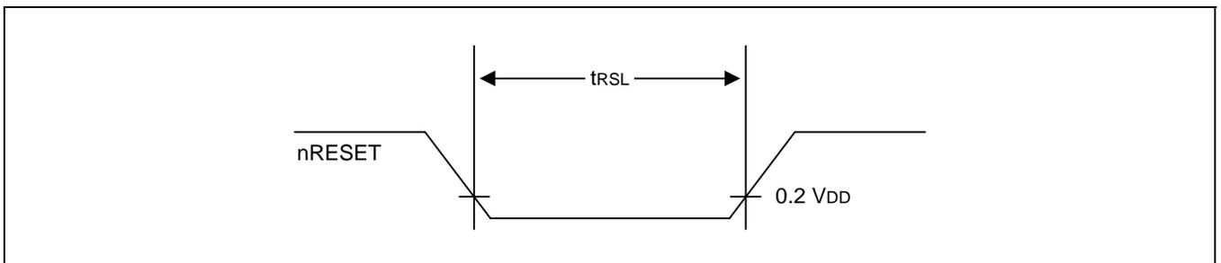
Figure 20-2. Input Timing for nRESET
