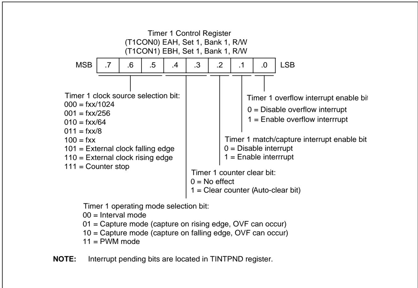
**Figure 12-1. Timer 1(0,1) Control Register (T1CON0, T1CON1)**
