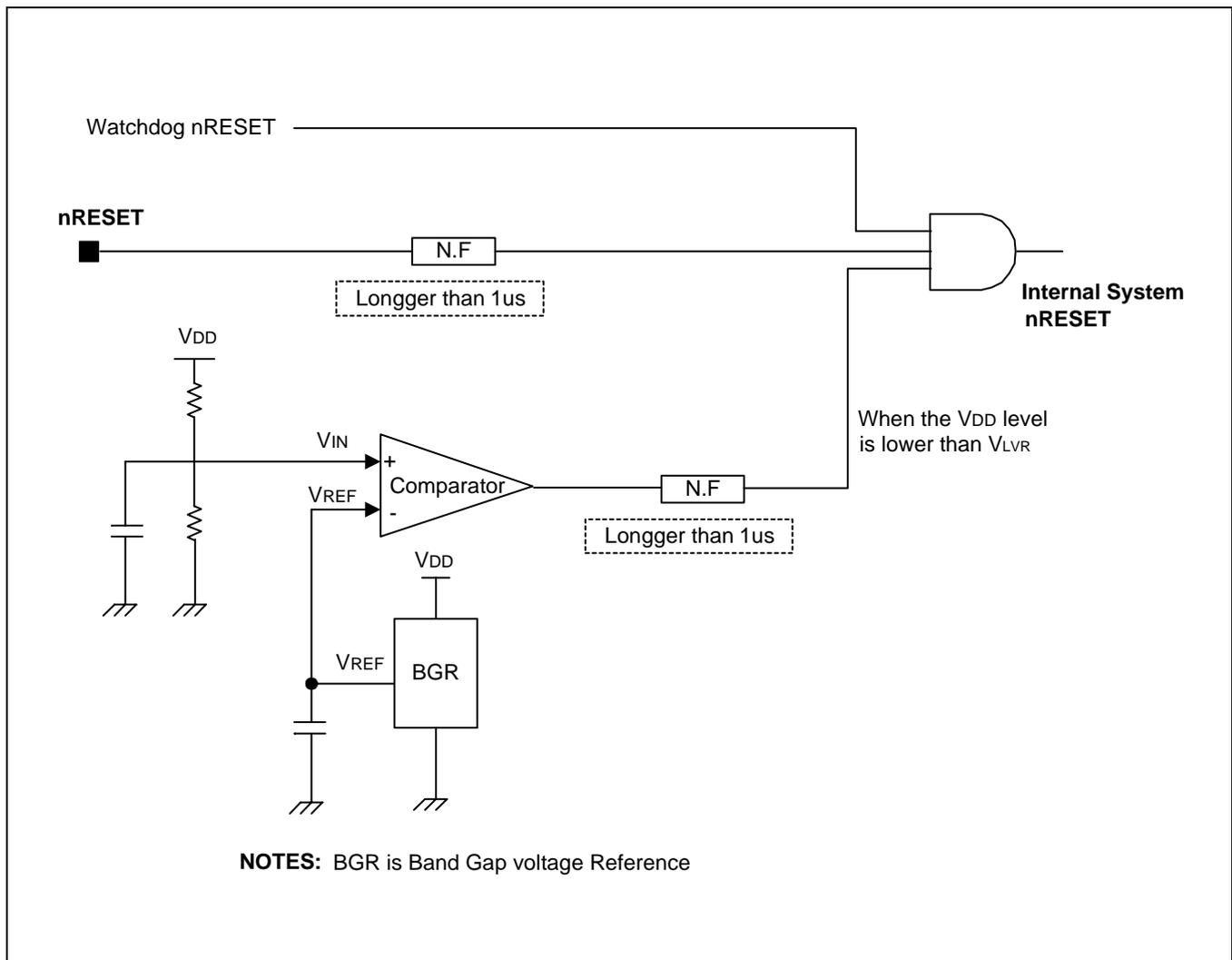
Figure 18-1. Low Voltage Reset Circuit
