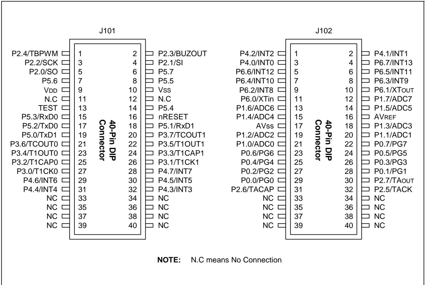
Figure 22-5. 40-Pin Connector Pin Assignment for TB84NB
