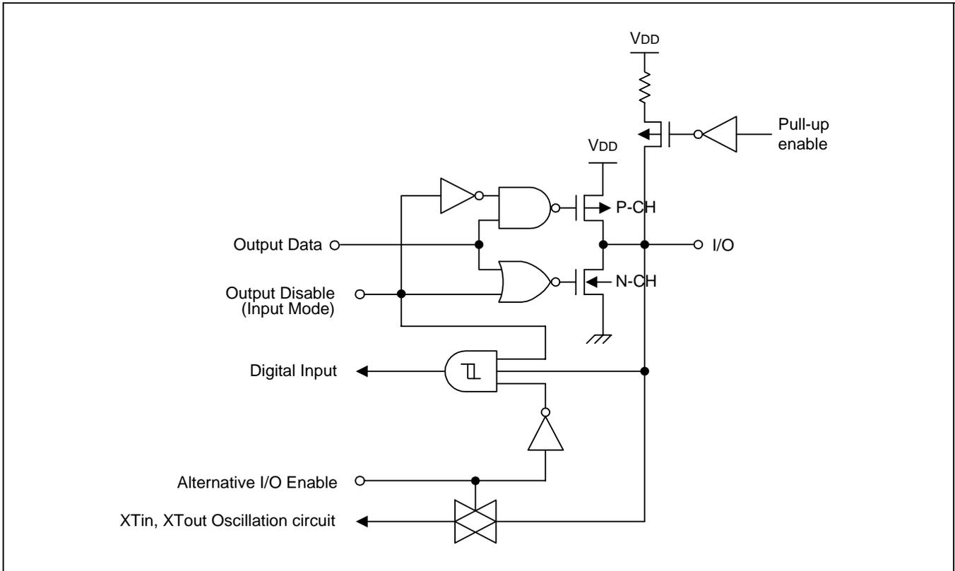
Figure 1-9. Pin Circuit Type F (P6.0, P6.1)
