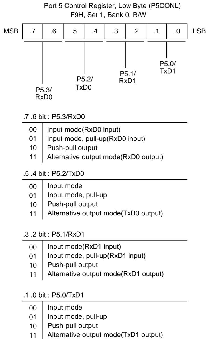
**Figure 9-13. Port 5 Low-Byte Control Register (P5CONL)**
