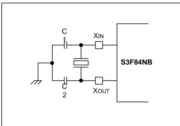
Figure 7-1. Main Oscillator Circuit
