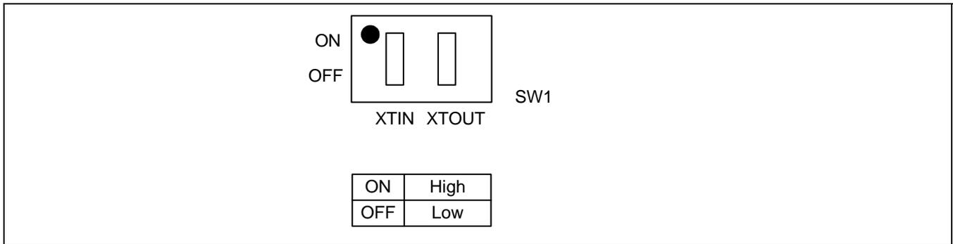
Figure 22-4. DIP Switch for Port 6 (Sub Oscillator or normal I/O)
