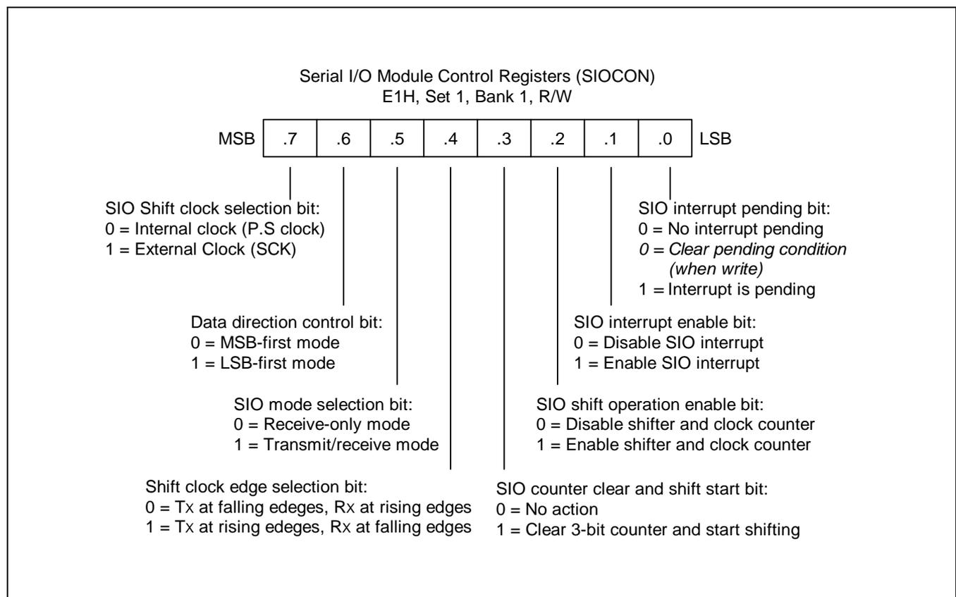
**Figure 13-1. Serial I/O Module Control Registers (SIOCON)**
