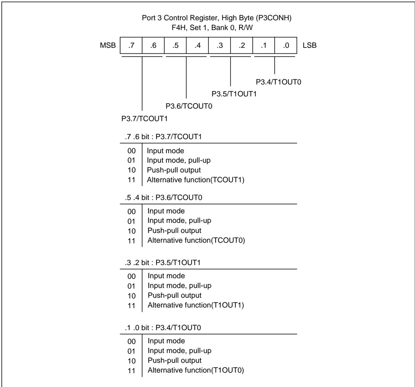
**Figure 9-6. Port 3 High-Byte Control Register (P3CONH)**
