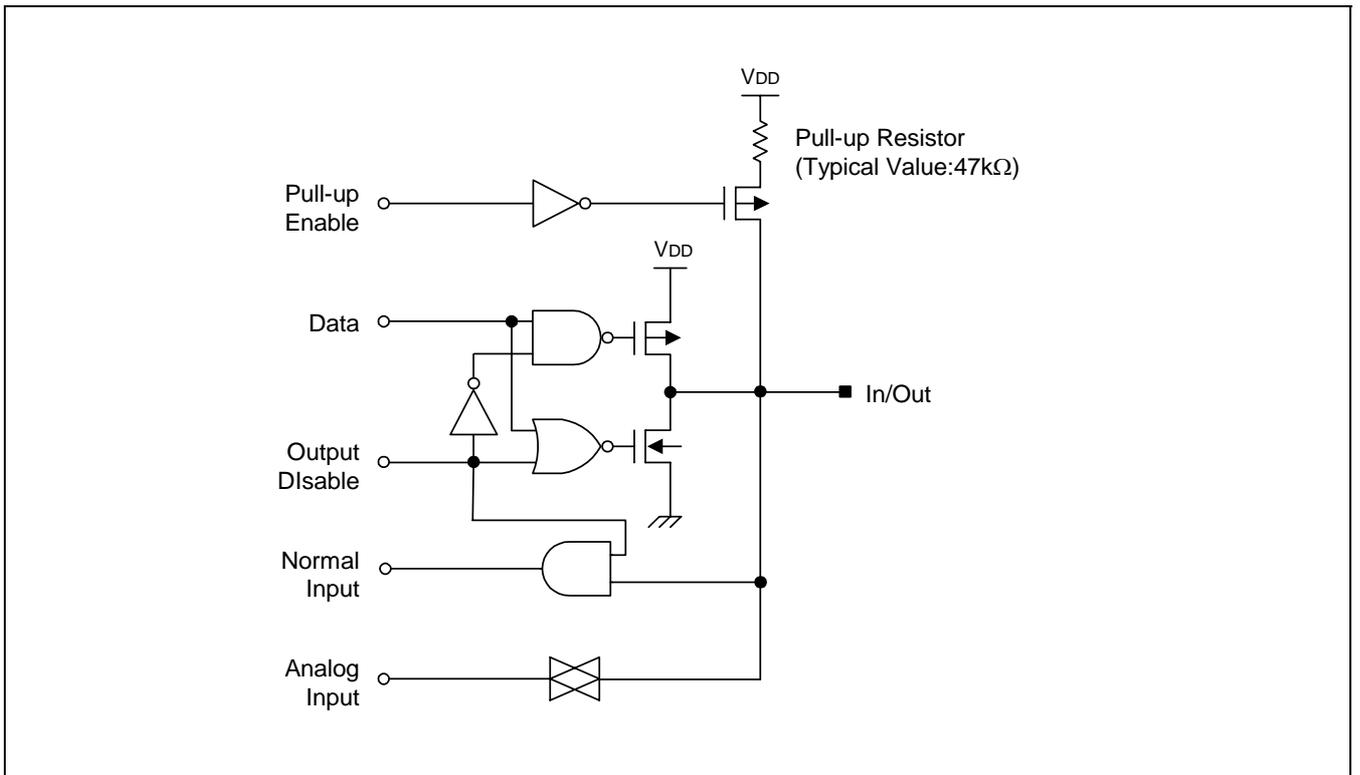
Figure 1-8. Pin Circuit Type E (Port 1)
