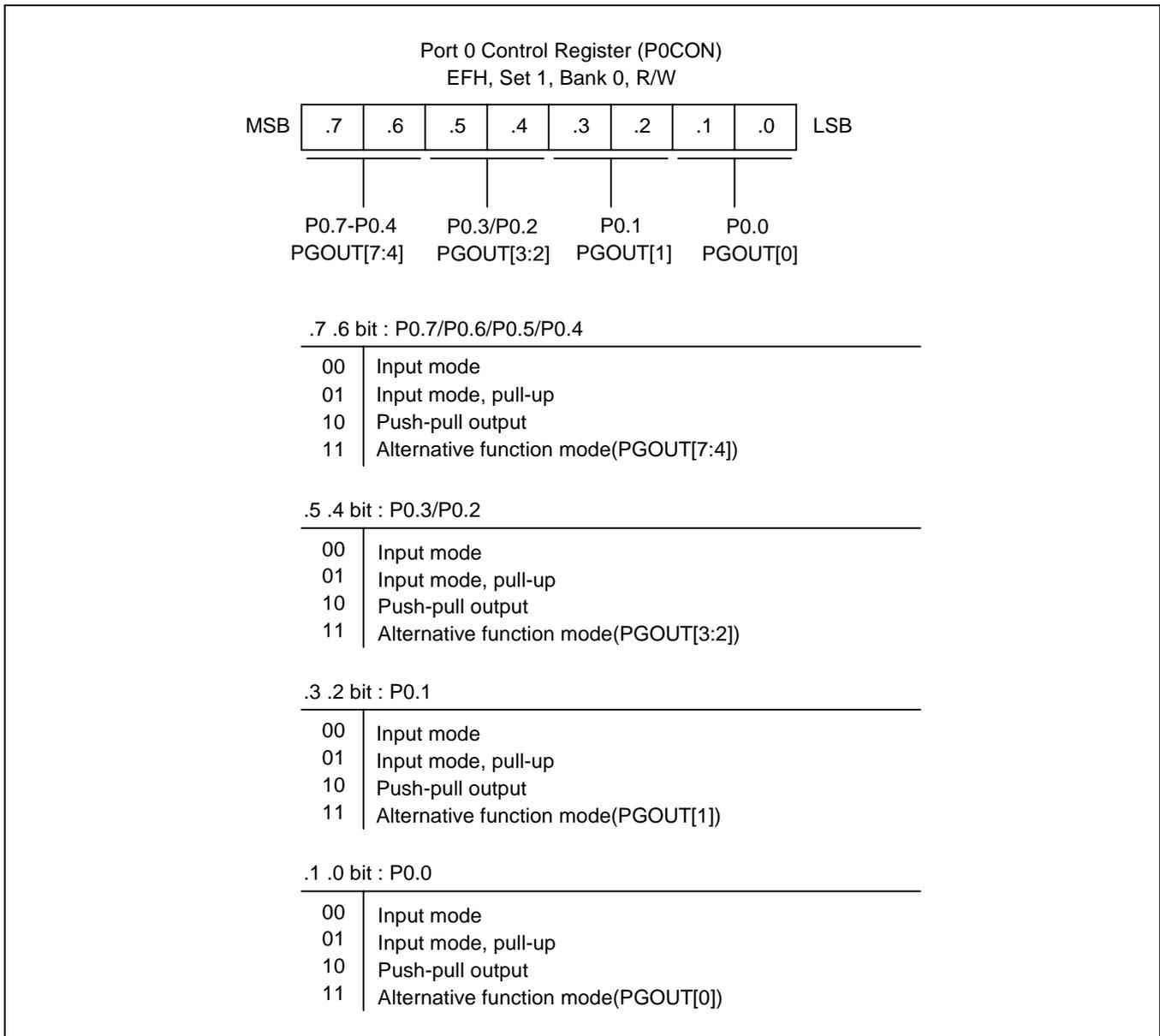
**Figure 9-1. Port 0 Control Register (P0CON)**
