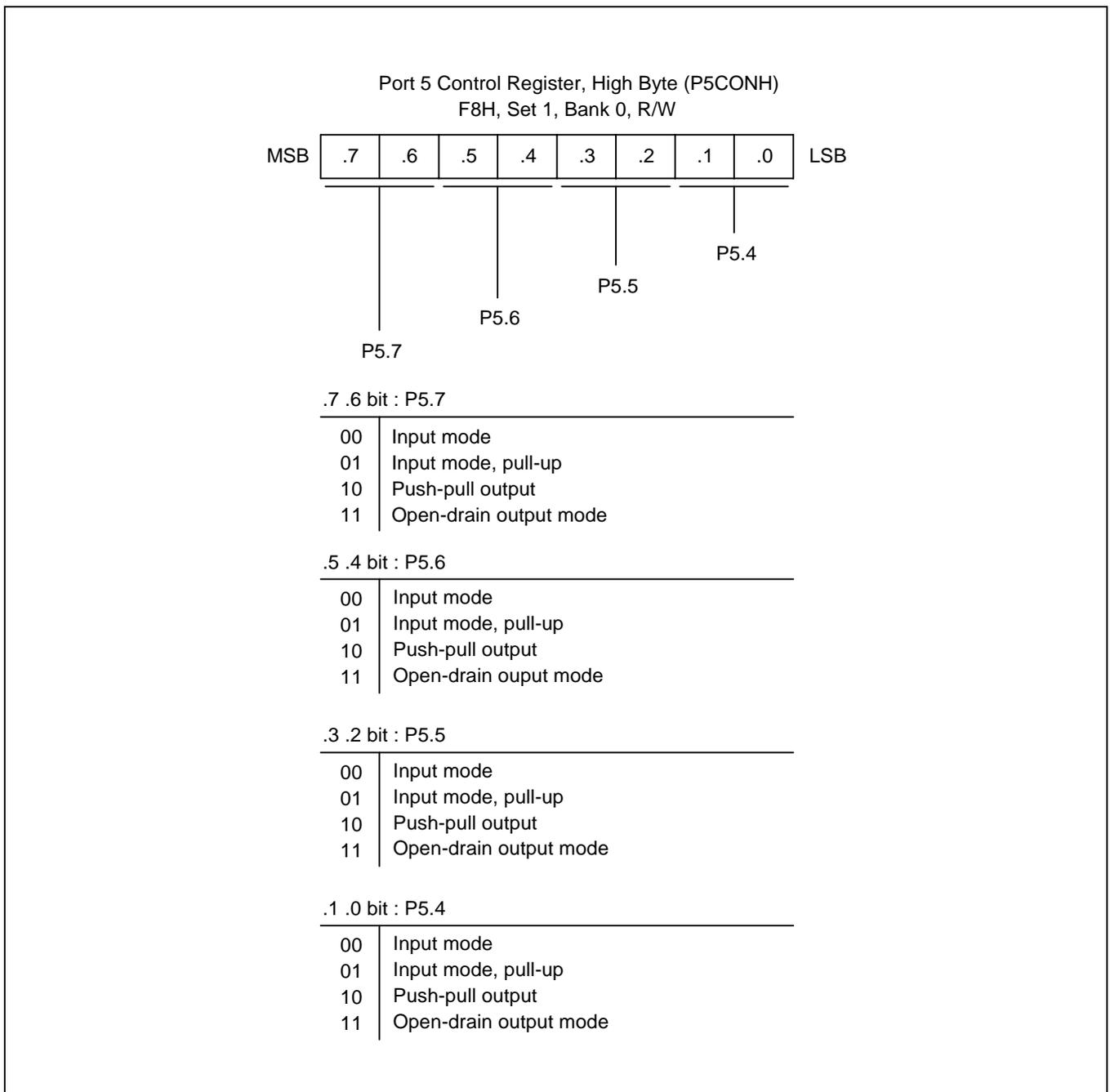
**Figure 9-12. Port 5 High-Byte Control Register (P5CONH)**
