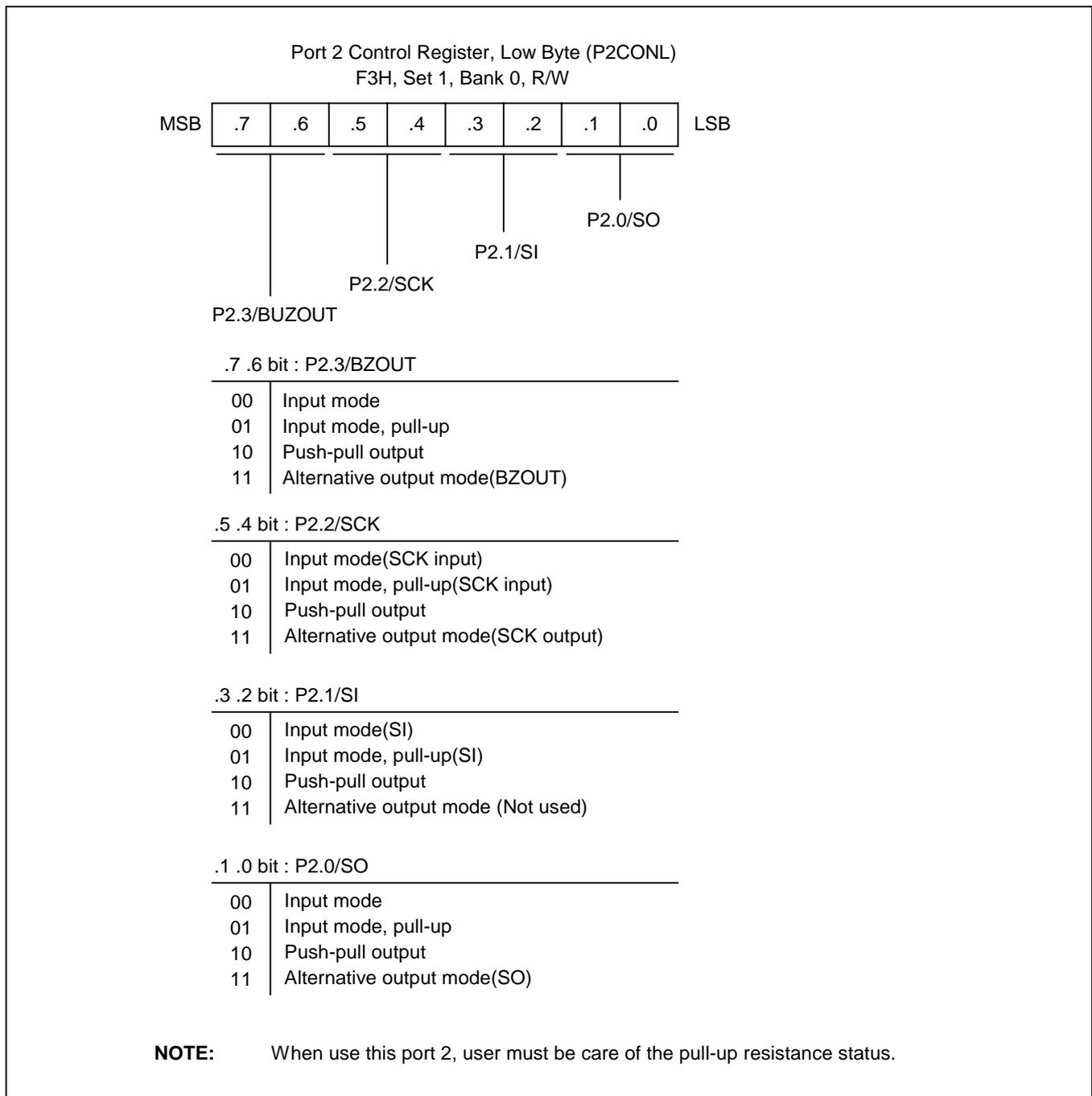
**Figure 9-5. Port 2 Low-Byte Control Register (P2CONL)**
