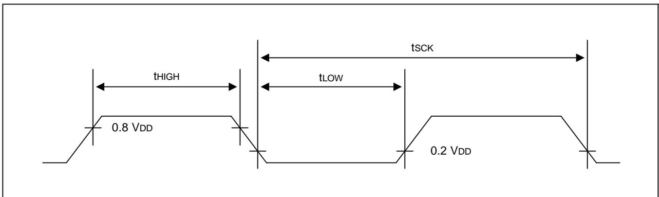
Figure 20-9. Waveform for UART Timing Characteristics
