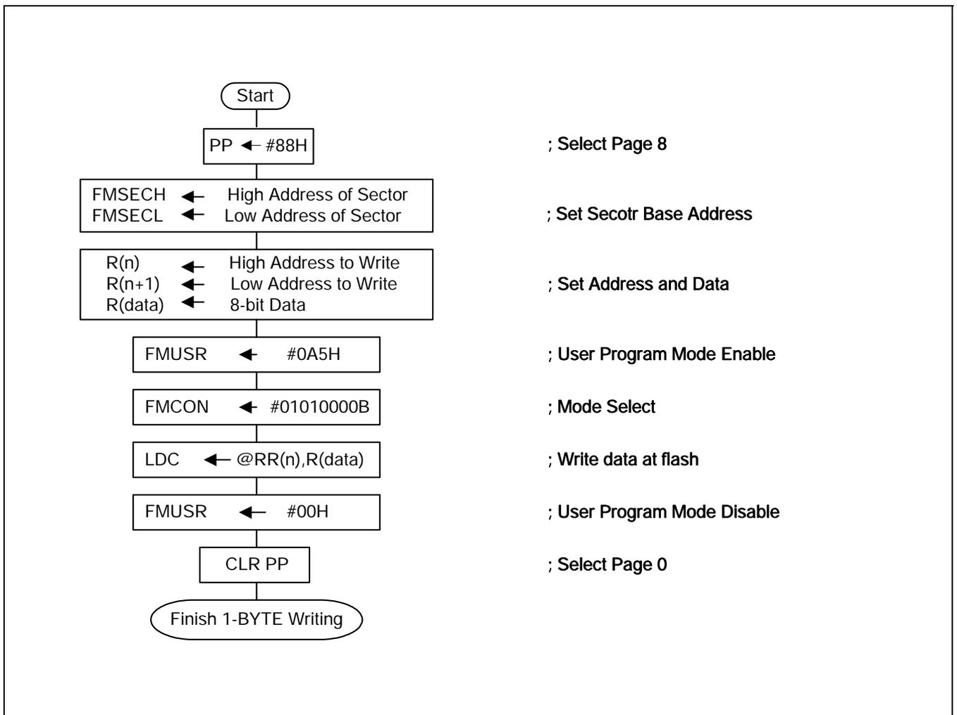
Figure 19-9. Byte Program Flowchart in a User Program Mode
