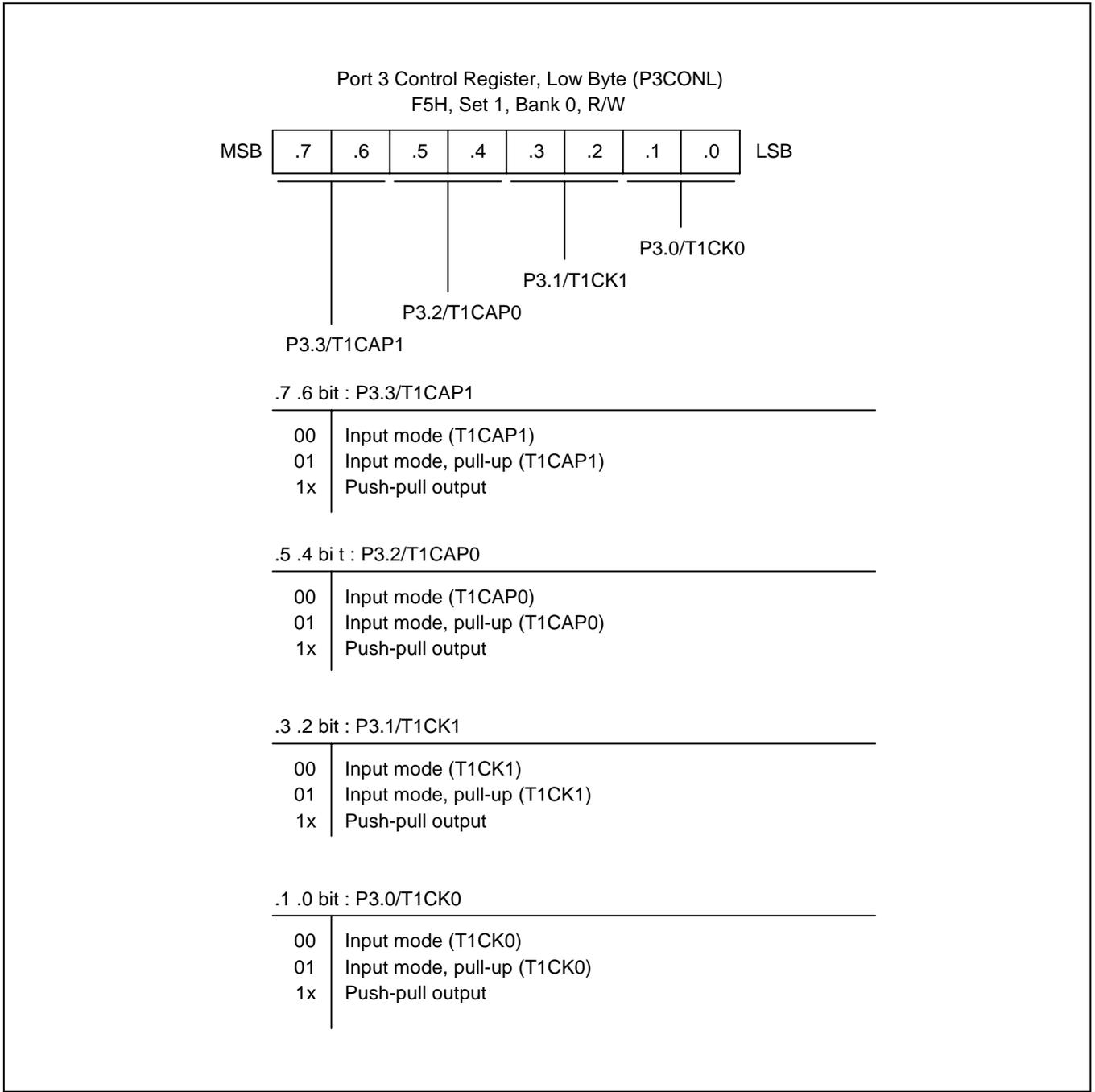
Figure 9-7. Port 3 Low-Byte Control Register (P3CONL)
