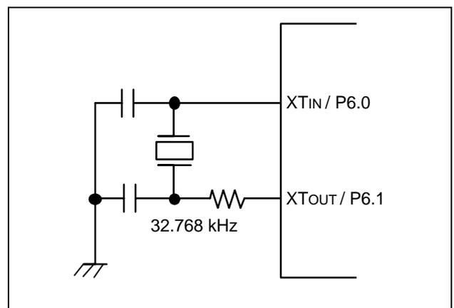
Figure 7-2. Sub-System Oscillator Circuit
