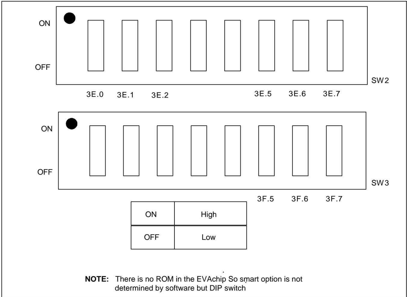
Figure 22-3. DIP Switch for Smart Option
