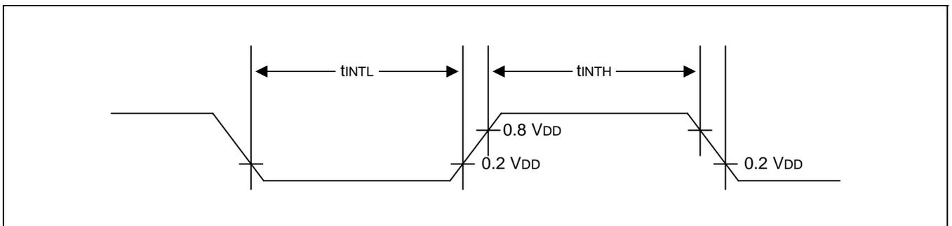
Figure 20-1. Input Timing for External Interrupts (Ports 4 and 6)
