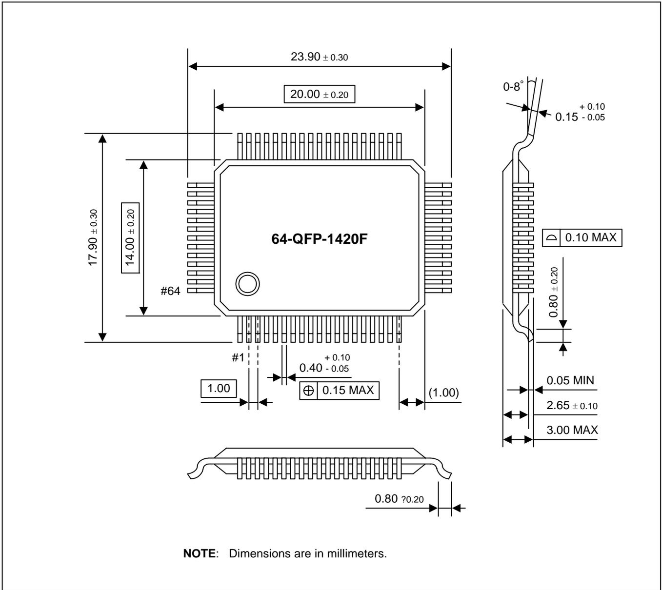
Figure 21-2. 64-QFP-1420F Package Dimensions
