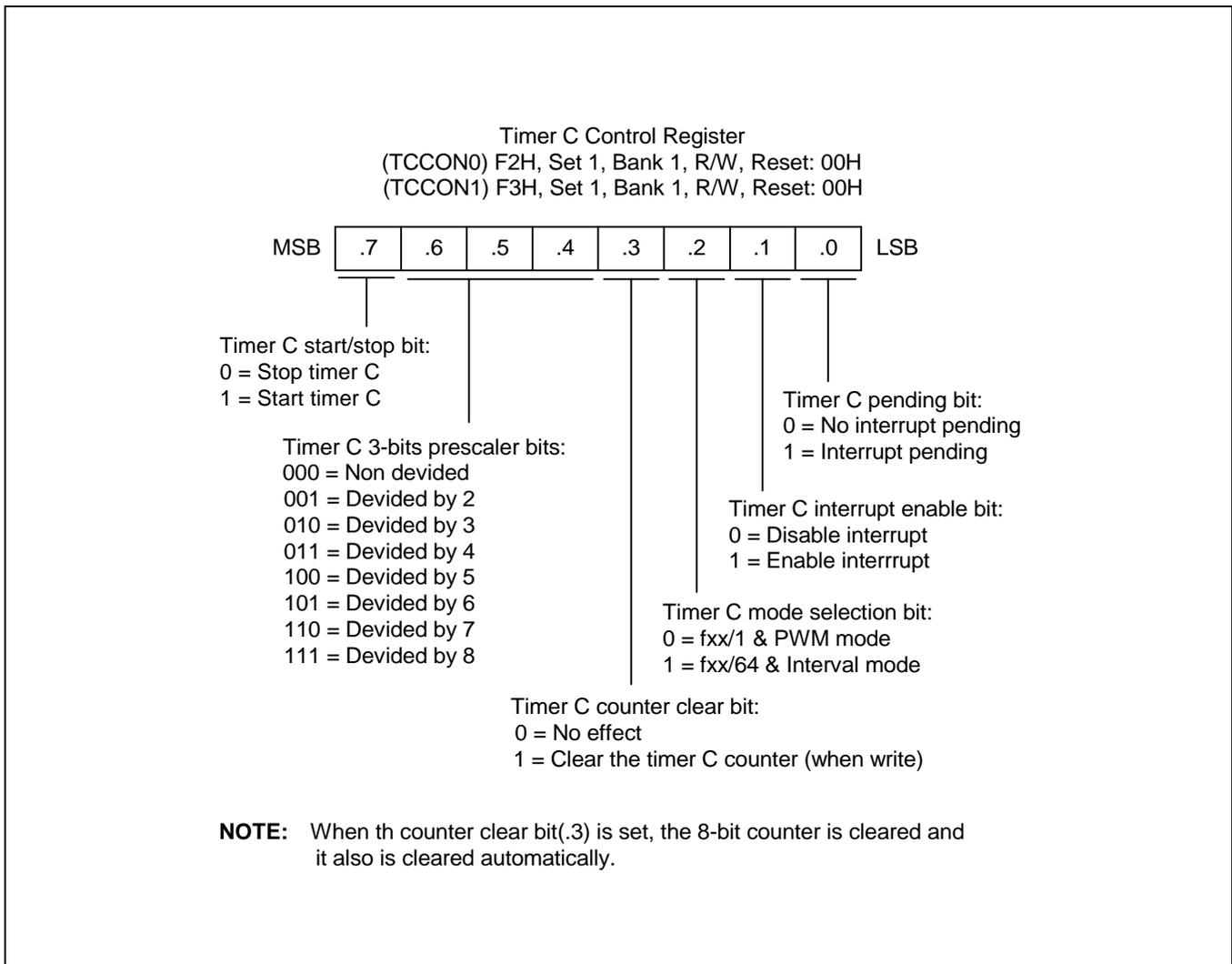
Figure 11-7. Timer C0, C1 Control Register (TCCON0, TCCON1)
