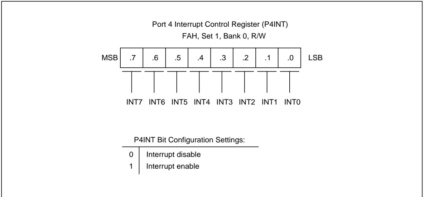
**Figure 9-10. Port 4 Interrupt Control Register (P4INT)**
