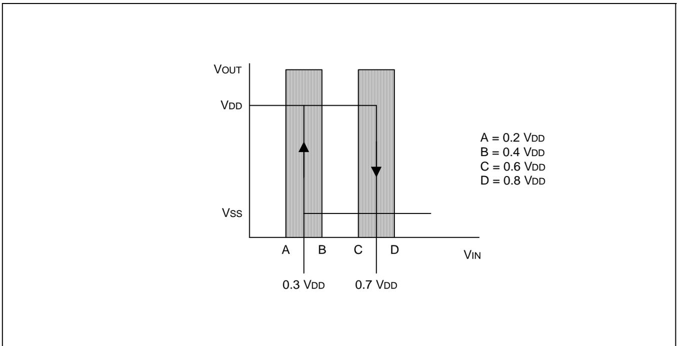
Figure 20-4. Schmitt Trigger Input Characteristics Diagram
