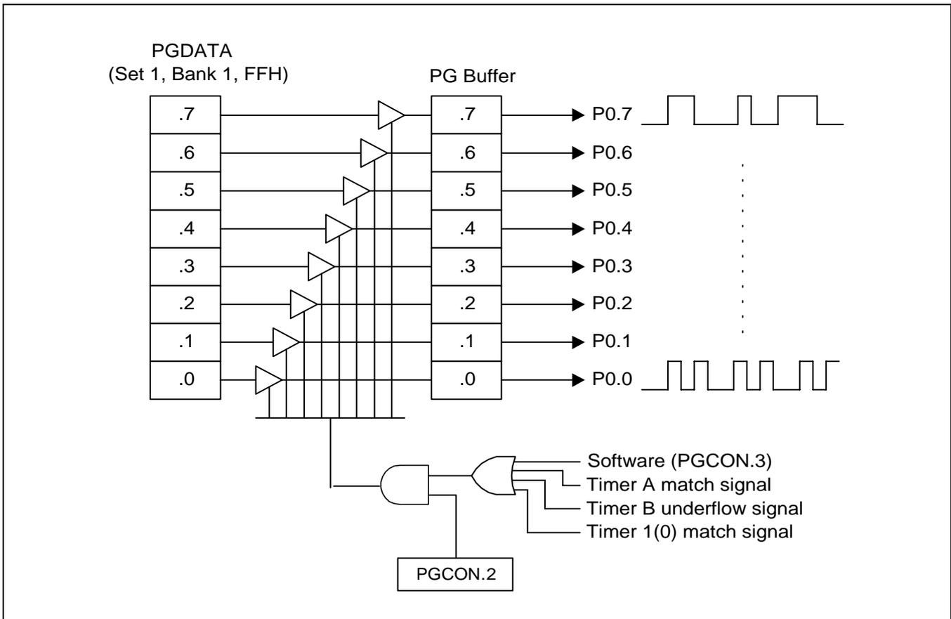
Figure 17-3. Pattern Generation Circuit Diagram
