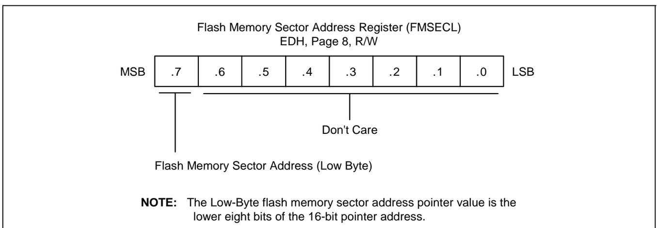
**Figure 19-6. Flash Memory Sector Address Register (FMSECL)**
