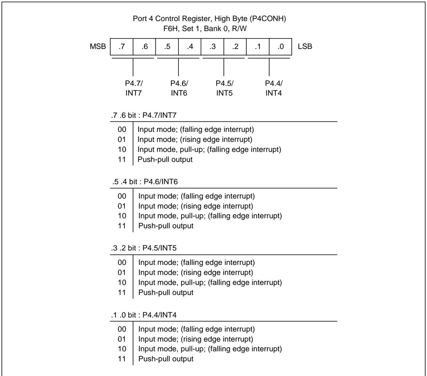
**Figure 9-8. Port 4 High-Byte Control Register (P4CONH)**
