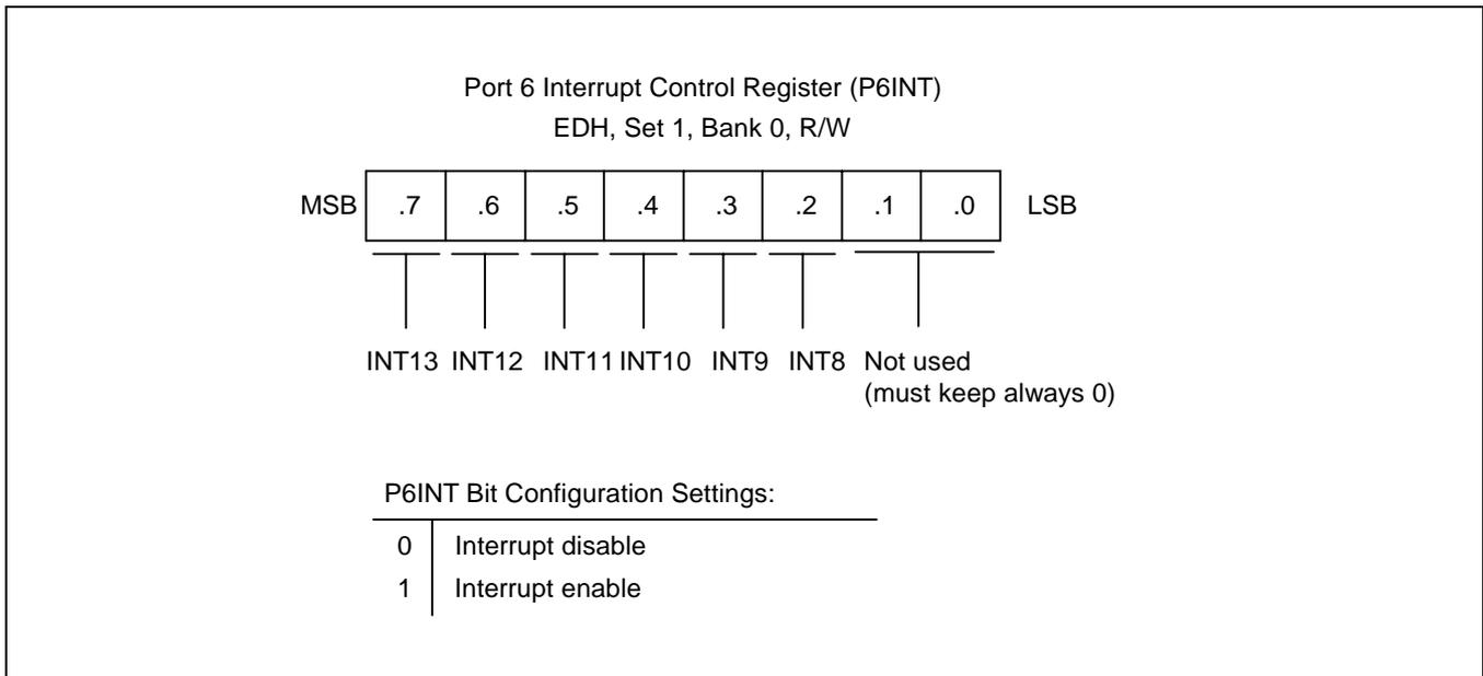
**Figure 9-16. Port 6 Interrupt Control Register (P6INT)**
