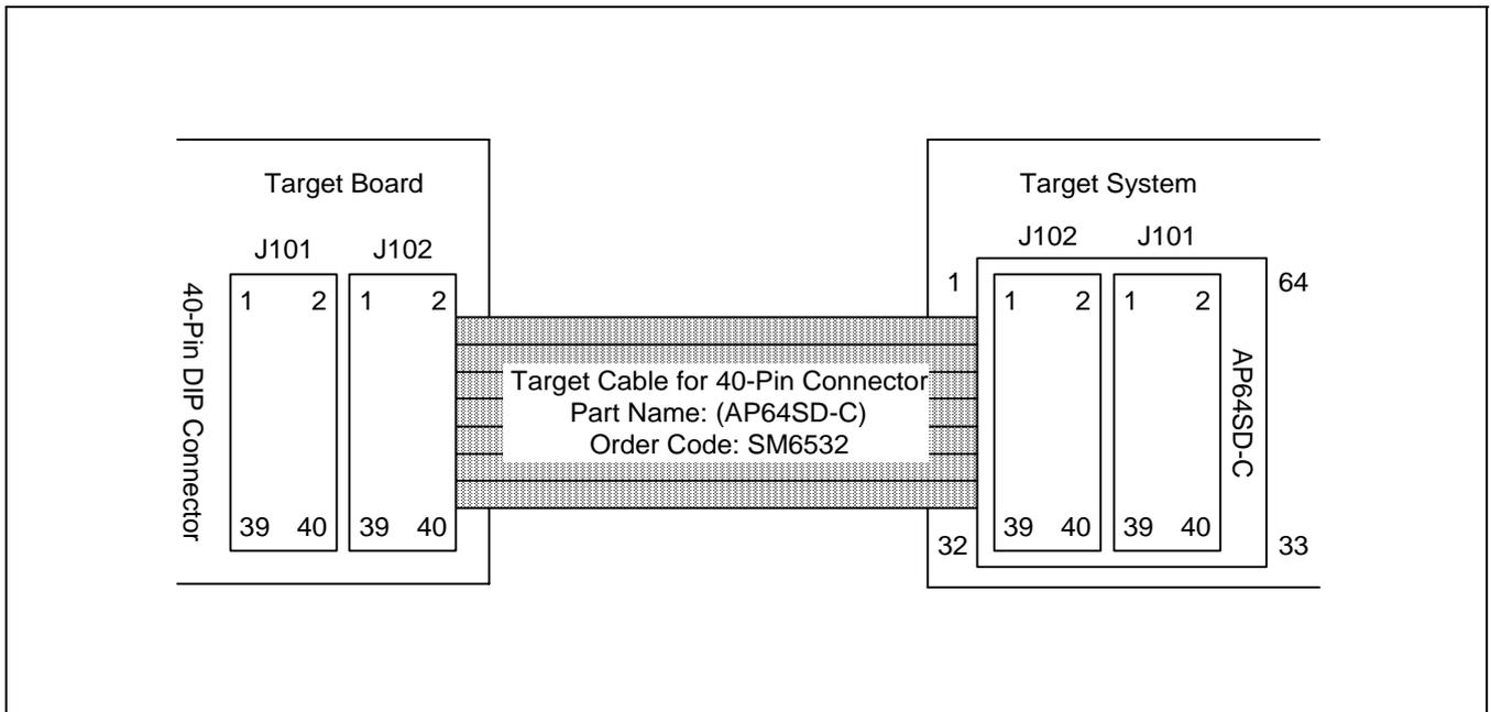
Figure 22-6. TB84NB Adapter Cable for 64-SDIP Package
