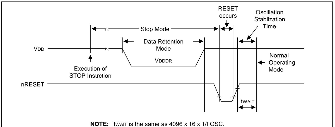
**Figure 20-5. Stop Mode Release Timing initiated by nRESET**
