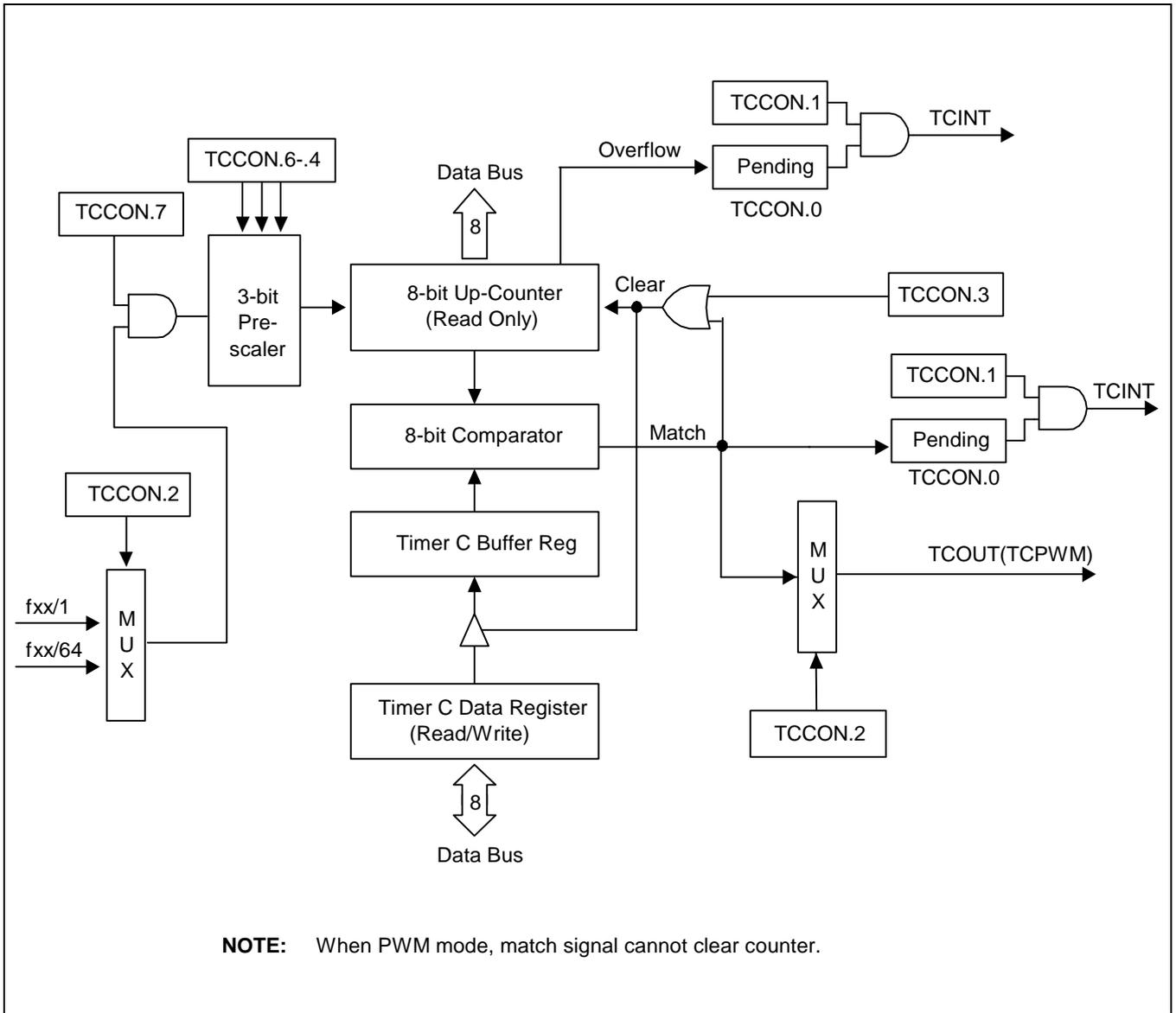
Figure 11-8. Timer C0, C1 Functional Block Diagram
