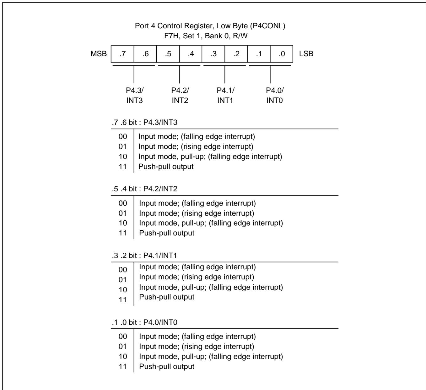
**Figure 9-9. Port 4 Low-Byte Control Register (P4CONL)**
