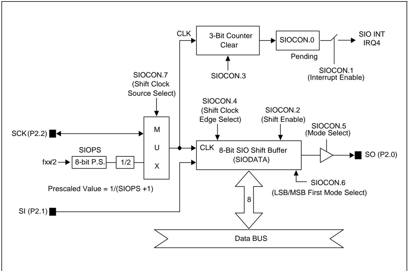
Figure 13-3. SIO Functional Block Diagram
