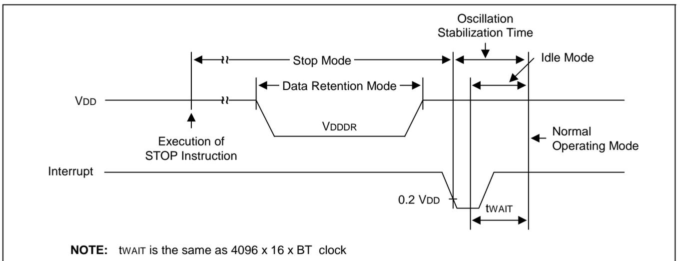
**Figure 20-6. Stop Mode (Main) Release Timing Initiated by Interrupts**
