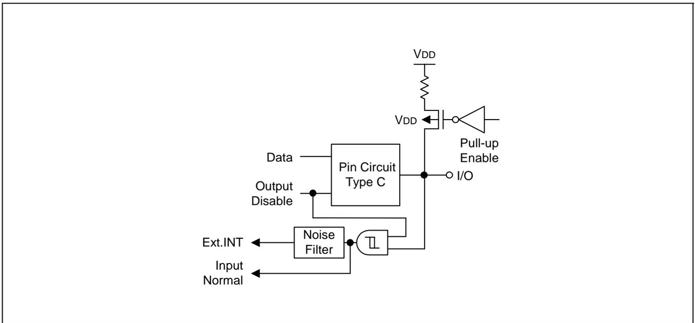
Figure 1-7. Pin Circuit Type D-1 (Port 4, and P6.2-P6.7)
