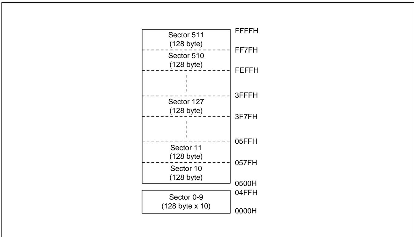
Figure 19-7. Sector Configurations in User Program Mode
