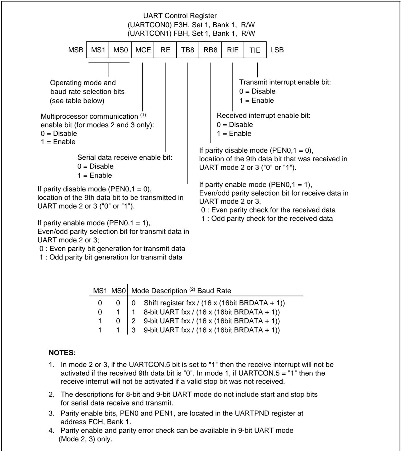
**Figure 14-1. UART Control Register (UARTCON0, UARTCON1)**
