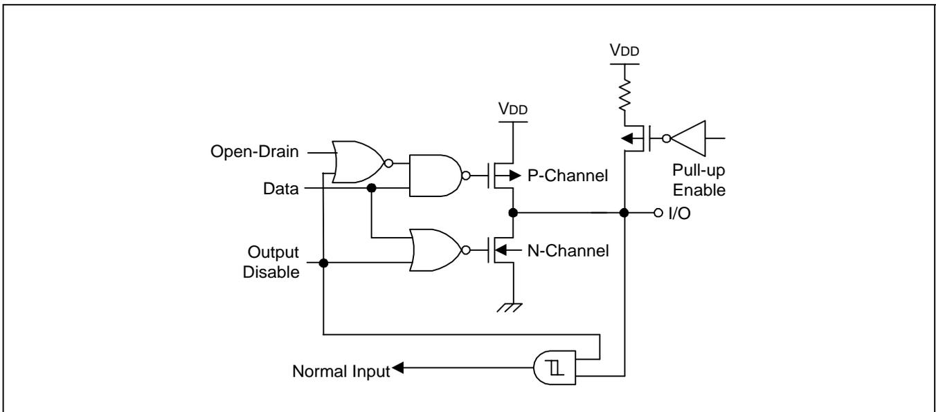
Figure 1-10. Pin Circuit Type G (P5.4-P5.7)
