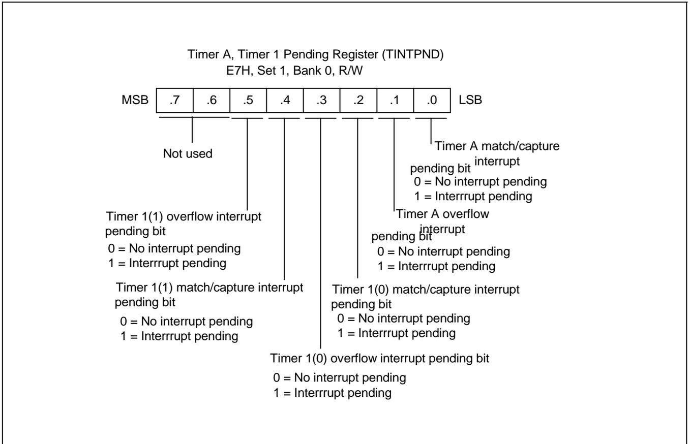
Figure 12-2. Timer A, Timer 1(0,1) Pending Register (TINTPND)
