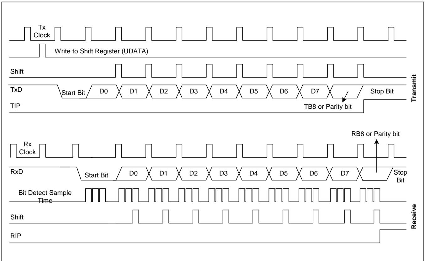
Figure 14-8. Timing Diagram for UART Mode 2 & 3 Operation
