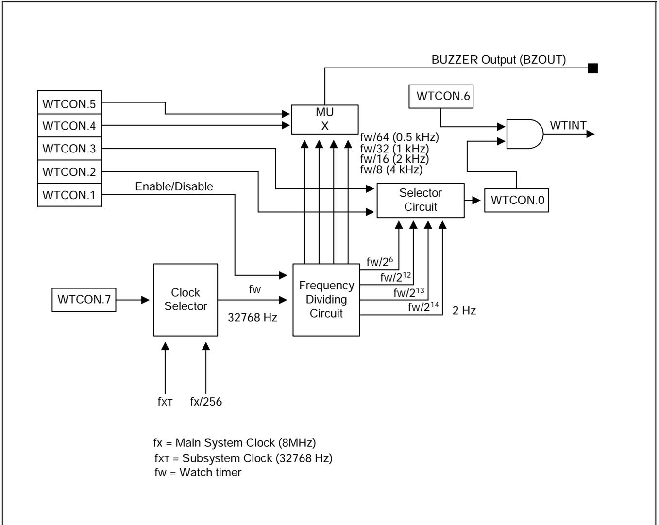
Figure 16-1. Watch Timer Circuit Diagram
