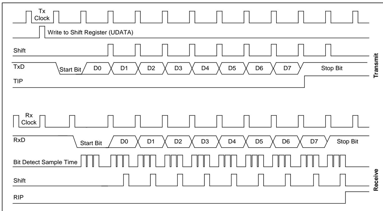
**Figure 14-7. Timing Diagram for UART Mode 1 Operation**
