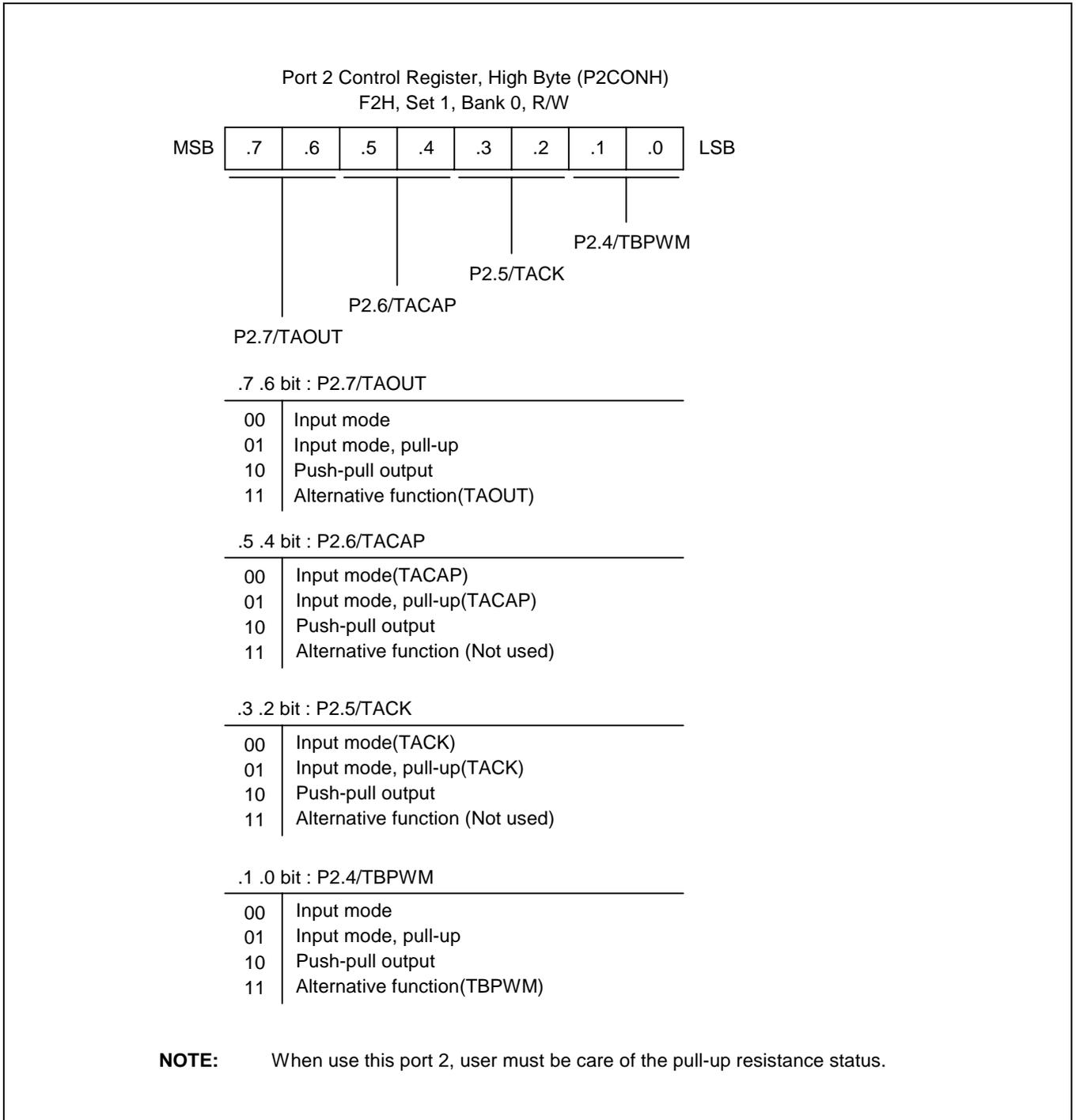
**Figure 9-4. Port 2 High-Byte Control Register (P2CONH)**
