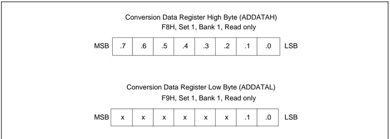
**Figure 15-2. A/D Converter Data Register (ADDATAH, ADDATAL)**
