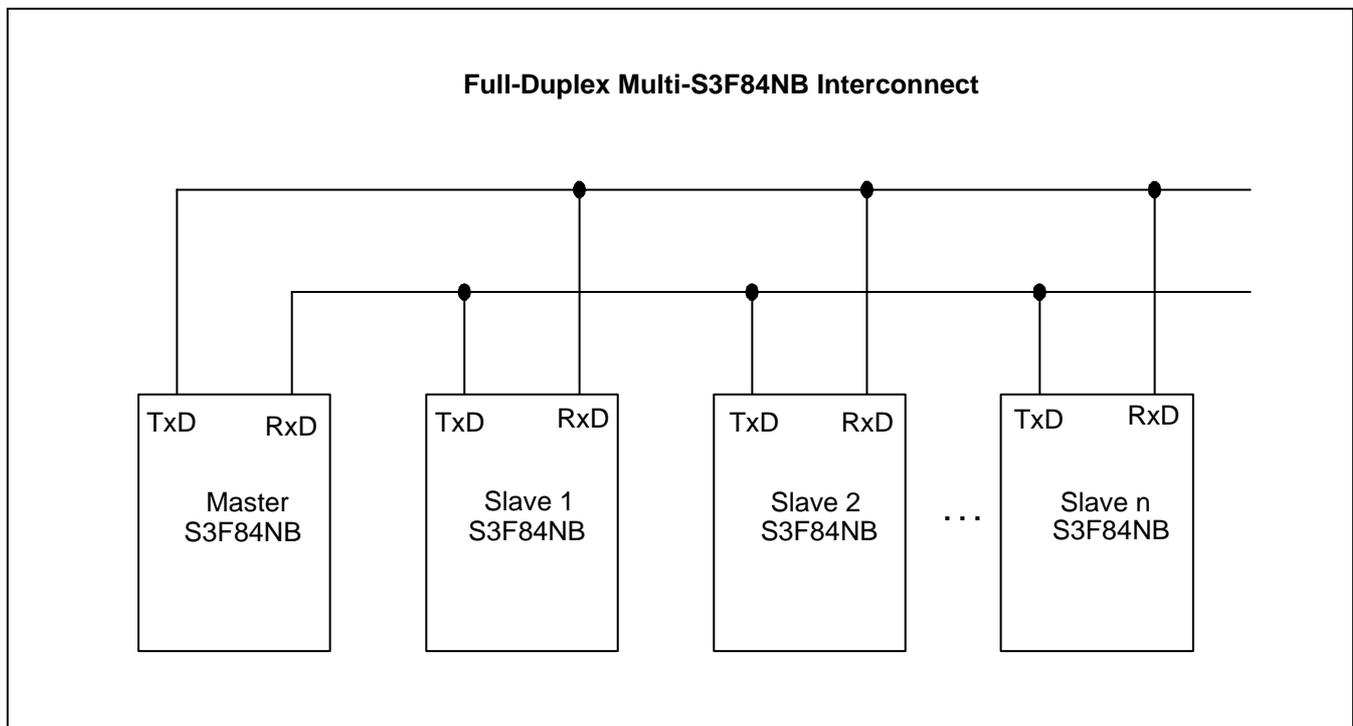
Figure 14-9. Connection Example for Multiprocessor Serial Data Communications
