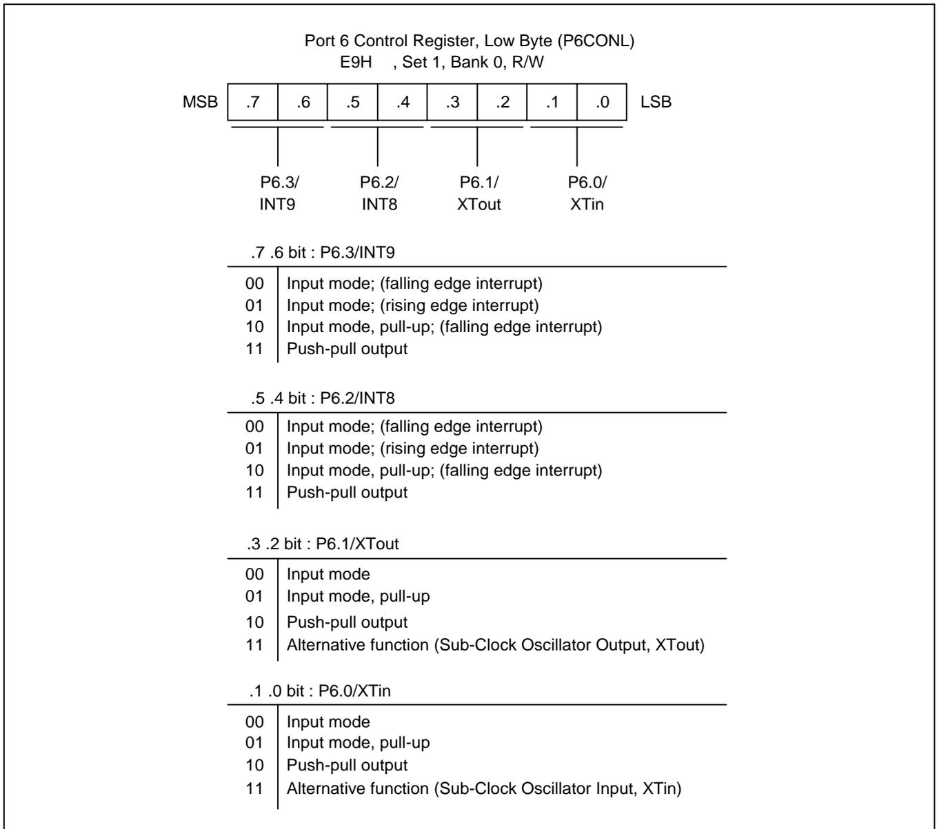
**Figure 9-15. Port 6 Low-Byte Control Register (P6CONL)**
