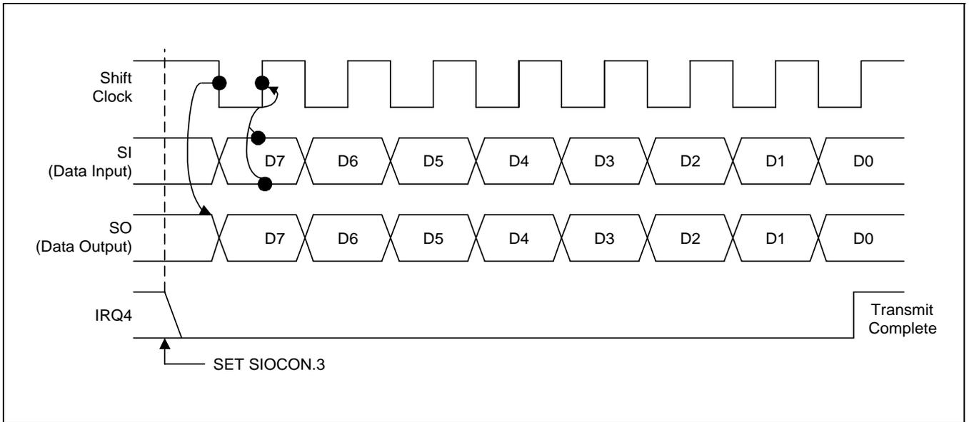
Figure 13-4. SIO Timing in Transmit/Receive Mode (Tx at falling edge, SIOCON.4=0)
