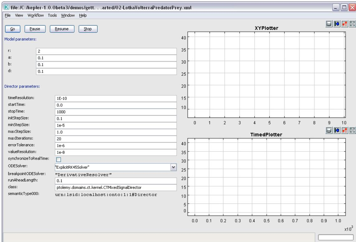
**Figure 9:** The Runtime window, displaying the Lotka-Volterra workflow. Click the Go button to run the workflow. Director and model parameters can be edited in the Runtime window. Output is displayed in the window as well.
