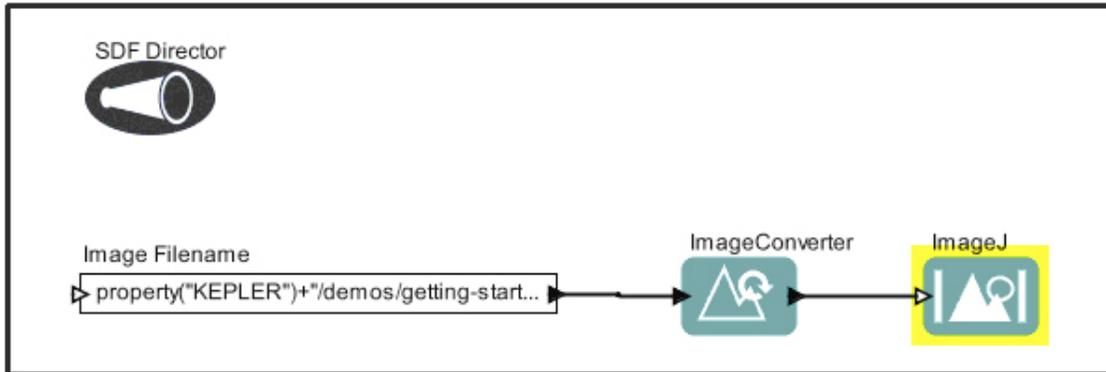
**Figure 14:** Image Display workflow showing *ImageJ* actor highlighted
