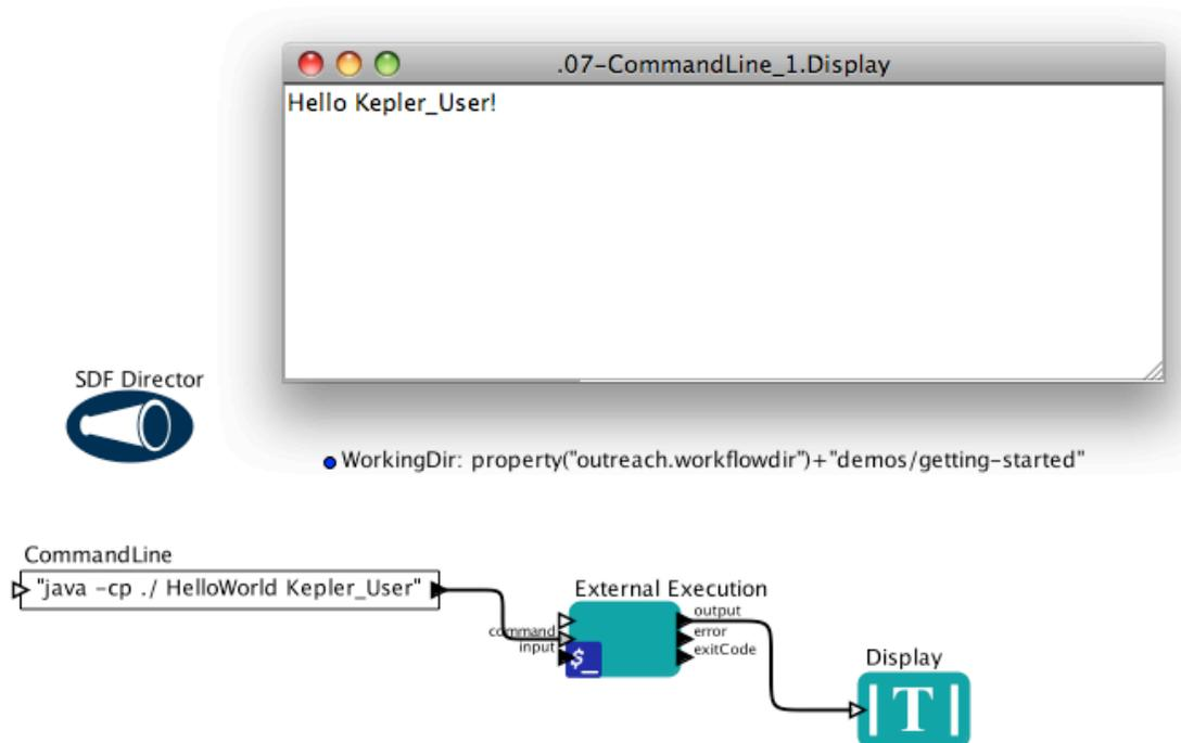
**Figure 34:** The Command Line workflow and its default output.
