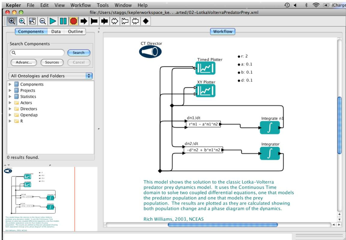
Figure 8: The Lotka-Volterra workflow in the Kepler interface.
