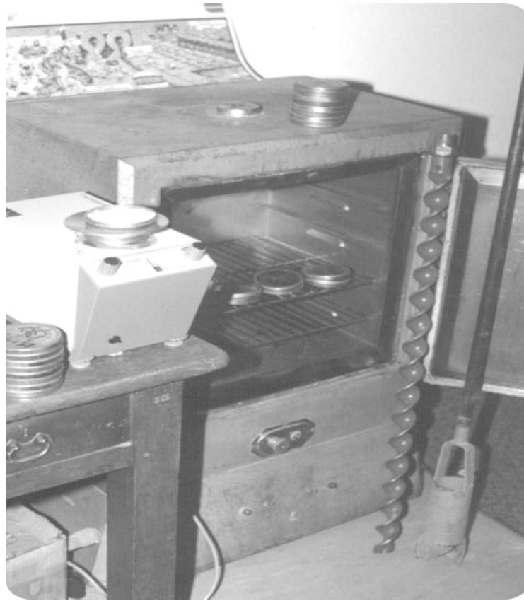
Figure 12.13: Apparatus required for the gravimetric method
