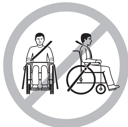
Incorrect placement of belt
