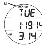
Fig. 2 - LOW BATTERY WARNING
