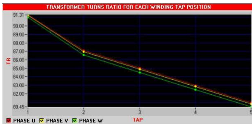
Figure 5-25: Graph showing the transformation ratio measured at the different regulator/adjuster positions.
