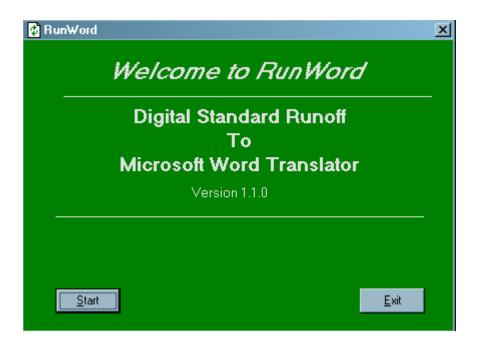
The <u>Start</u> button will open the file dialog box. Selecting a file and pressing the <u>Open button will start</u> the conversion process.
