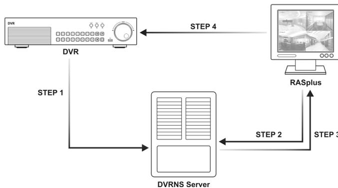
**STEP 1 (DVR → DVRNS Server):** Register the unit name and IP address of the DVR during the DVRNS setup on the Remote DVR. This unit name and IP address will be registered on the DVRNS server directly.
