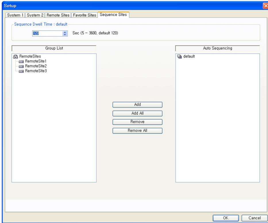
**Sequence Site:** Configure the sequence site. RASplus connects to the registered sites sequentially allowing connection to more than one remote site. Register an Auto Sequencing group and add desired sites in the Group List to the Auto Sequencing group. Video from the sites added to the Auto Sequencing group is displayed on the screen in the preset sequence interval during the sequence monitoring.
