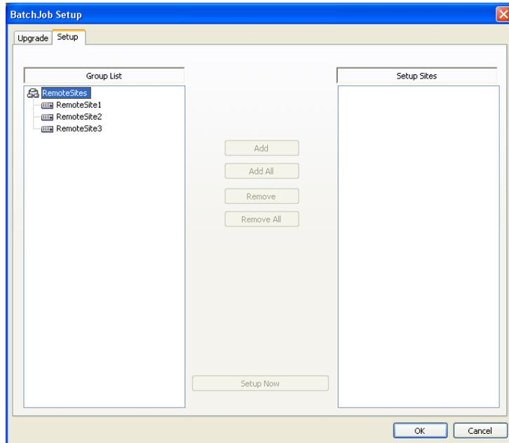
**Setup:** Imports saved settings from a remote DVR to the remote DVR. First, select the remote sites to set up from the Group List, and add them to the Setup Sites list by clicking the **Add** button. Then, click the **Setup Now** button to initiate the remote setup job for Setup Sites.
