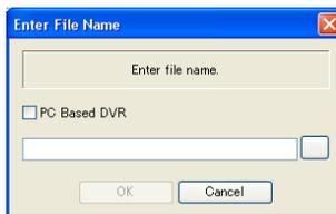
**NOTE:** When upgrading a PC-based DVR, select *PC Based DVR* and then select the desired upgrade folder.
