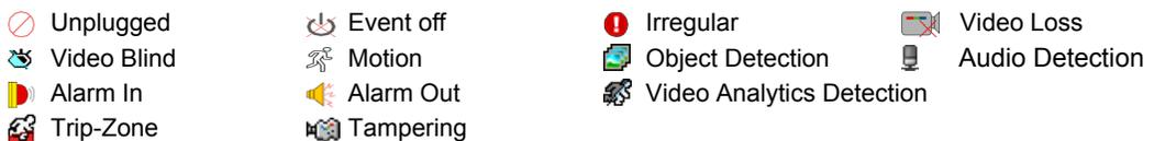
**NOTE: The device status is displayed as Irregular based on to the system check settings and as each event according to the event detection settings on the remote DVR.**
