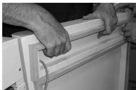
Figure 6-15. Install Top Pan & Gasket
