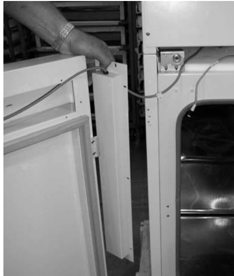
Figure 6-11. Set Door and Pan Aside
