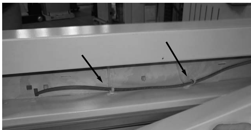
Figure 6-10. Release Tie Wraps
