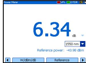
**Note:** The reference value you set for each wavelength remains in memory until a new one is set for the same wavelength, even when you turn the unit off.
