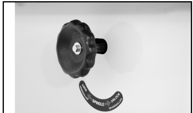
Figure-5 Loosening the spindle lock knob
