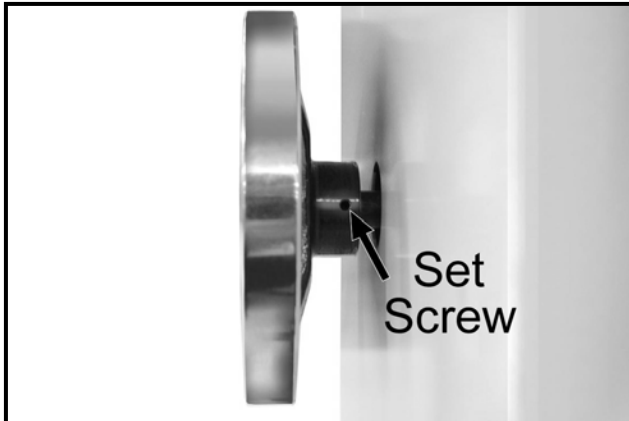
Figure-2 Securing the spindle height hand wheel
