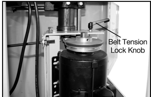
Figure-15 Loosening the belt tension
