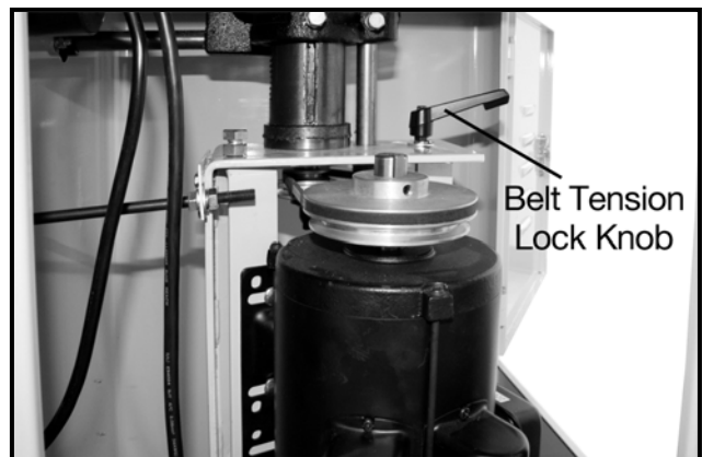
Figure-18 Belt tension lock knob
