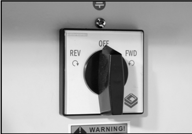
Figure-17 Forward / OFF / Reverse switch
