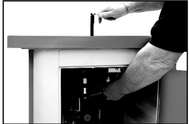
Figure-8 Installing the spindle
