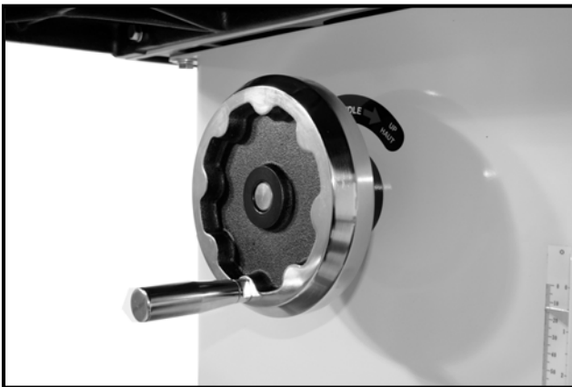
Figure-3 Installing the handle
