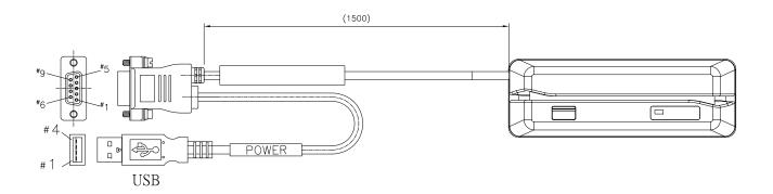
The DB-9F side of RS232 cable connects to PC COM port (COM 1 or COM 2 or other COMs) , and power connects to USB .
