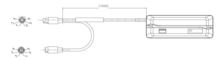
The MD-6M side of KB cable, shall be connected to PC PS/2 Keyboard port.
