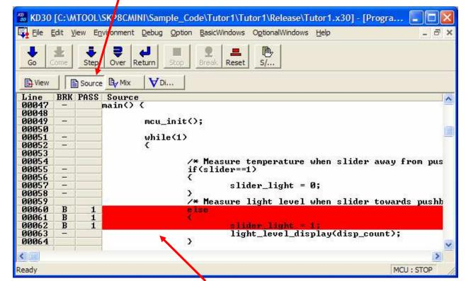
2. Locate and then set a breakpoint on 'else' in main() by a double-click on '-' in the 'BRK' column that denotes an executable line. A 'B' will appear in its place after the breakpoint is set and the line(s) is highlighted in red.
