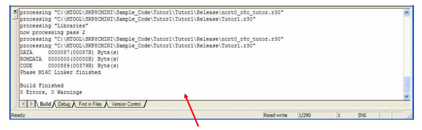
The no. of errors and warnings will show up in this window. You can then scroll up to find where the error(s) occurred. If no errors or warnings were found, 'Build Finished' will be displayed.
