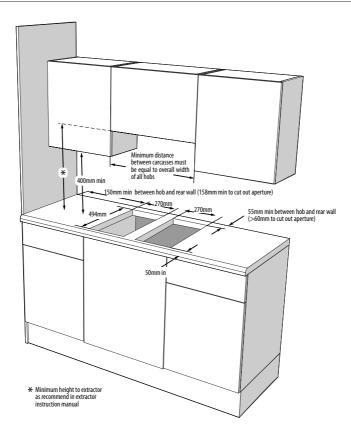
No shelf or overhang of combustible material should be closer than 650mm directly above the hob.
