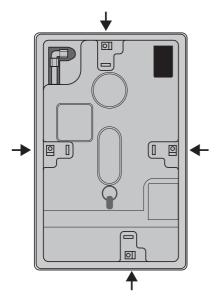
The two brackets are secured directly into the base of the hob in appropriate positions as shown.
