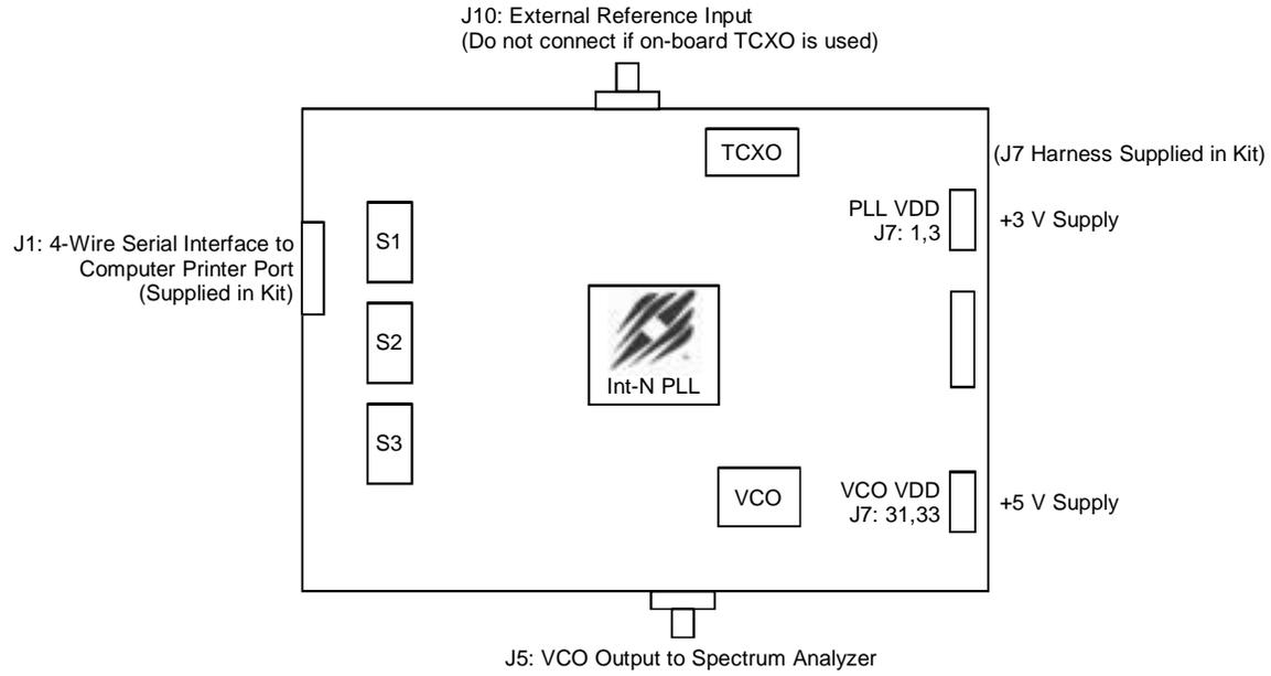
**Figure 2. Evaluation Kit Default Jumper & Switch Settings.**
