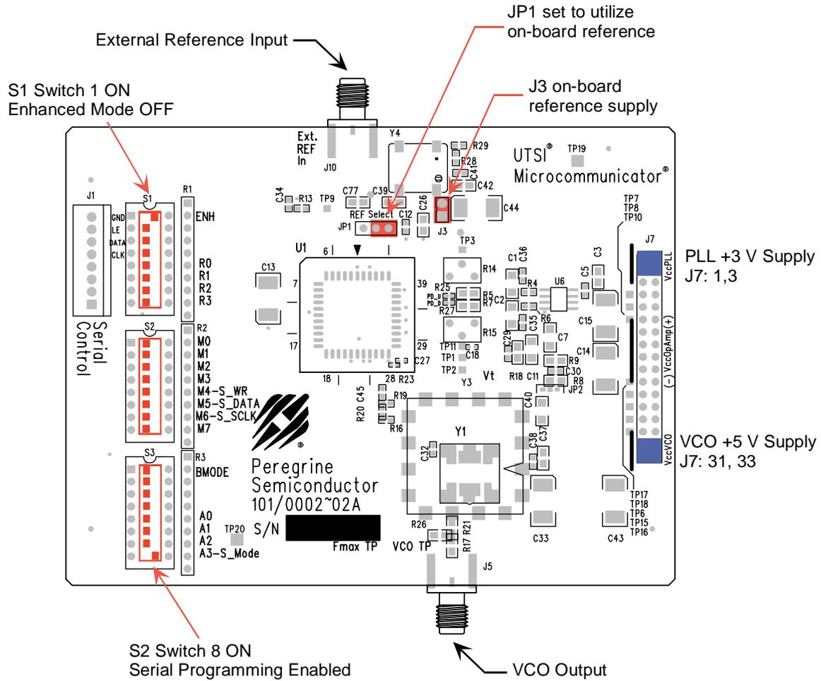
**Figure 3. Jumper Setting to Disable On-board Reference.**
