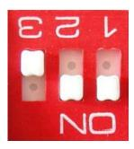
This mode is Safe mode. If any one of the two HDD in the dual bay docking gets bad, you can replace it with a new HDD. The dual bay docking will rebuild all files in the new HDD.
