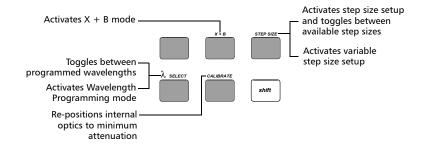
To access a secondary function, press shift, then the corresponding key. Note:
