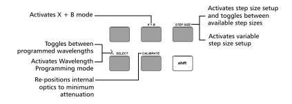
To access a secondary function, press shift, then the corresponding key. Note:
