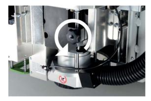
Release the lock to allow the suction house moving down to its down position.
