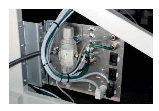
If a bit is stuck in the chuck, the probable cause is low air pressure.
