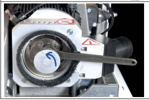
Hold the rotor with the 13 mm (17 mm for MultiCUT-HP) key and unscrew the chuck with the chuck tool.
