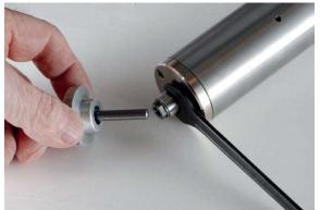
Enter the chuck tool with a dummy bit to the chuck.
