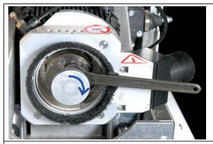
Torque up the chuck by hand, using the chuck tool and a dummy bit. (Maximum torque 2 Nm, 18 lbf-in). Hold the rotor with the 13 mm/17 mm key.
