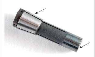
Apply small quantities of grease to the threads of the chuck when necessary. Avoid the clamping area. Do not use oil, as it could enter the clamping area and reduce the clamping force. Also apply small quantities of grease to the outer cone of the chuck.
