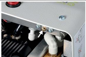
Push the air clean button to help remove contamination.
