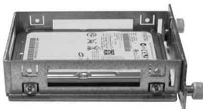
Fig. 25: Removed HDD tray with installed HDD (SATA0)
