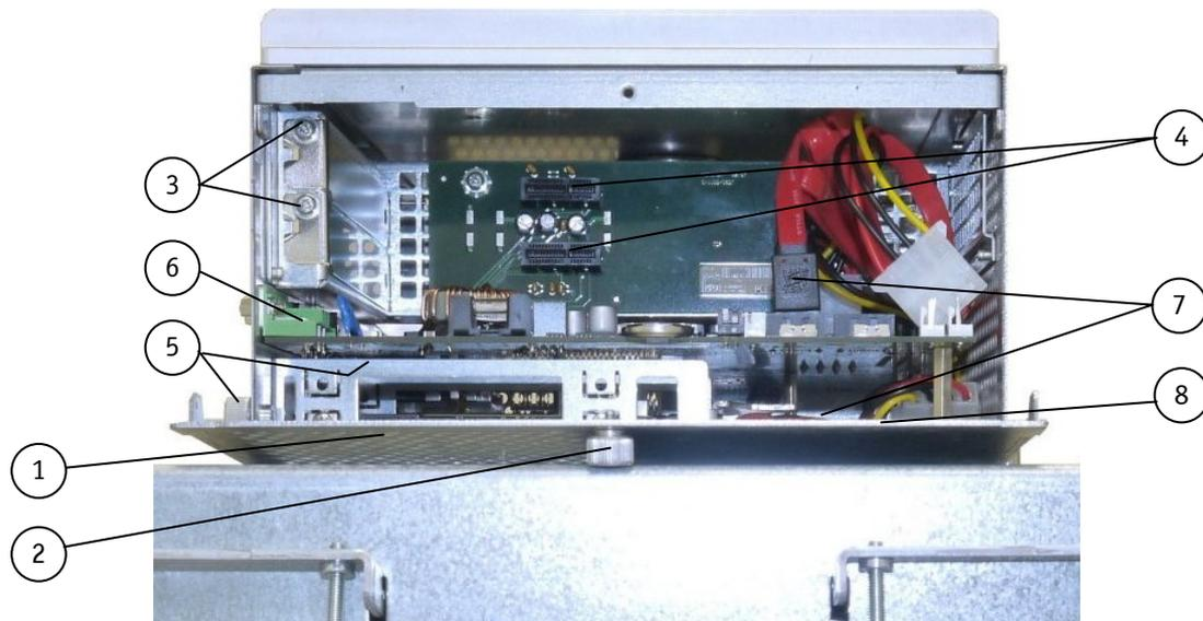
Fig. 19: Opened access door (system is shown with riser card for up to 2x PCIe x1 expansion slots)
