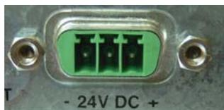
Fig. 33: DC-connector (without Phoenix plug terminal)
