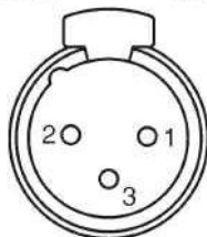
DMX - output XLR mounting-sockets (rear view):
