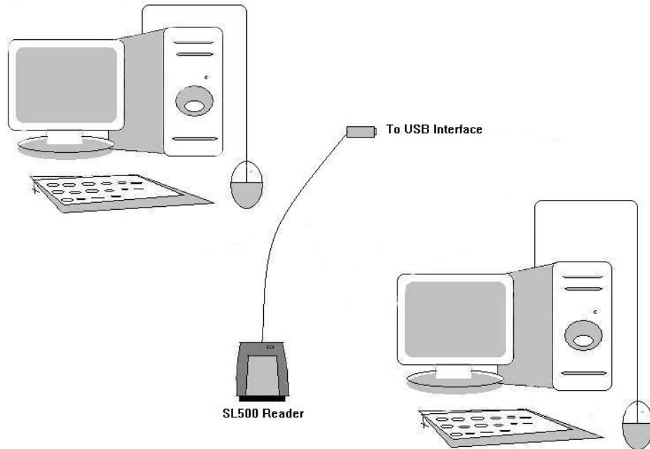
SL500-USB Reader is USB bridge to COM. Connect SL500 to the USB port of PC, after installing the driver will come out a virtual COM, the operations hereafter are as same as SL500-RS232.
