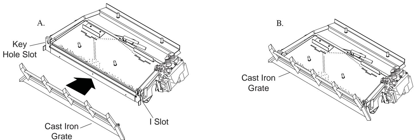
Figure 29 (a&b) - Installing Cast Iron Grate
