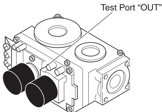
**Figure 16 - Pressure Test Point Location
