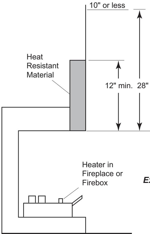
**Example:** The bottom of the mantel may project from the wall a maximum of 10" at a minimum of 28" above the opening.
