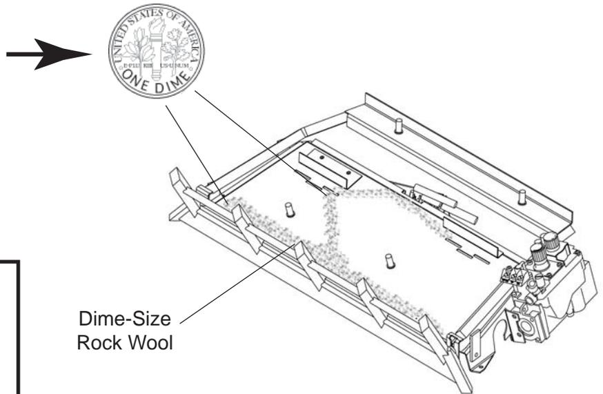
Figure 19 - Placing Rock Wool
