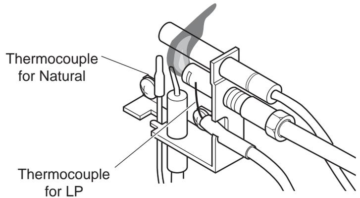
**Figure 31 - Incorrect Appearance of Pilot Flame**
