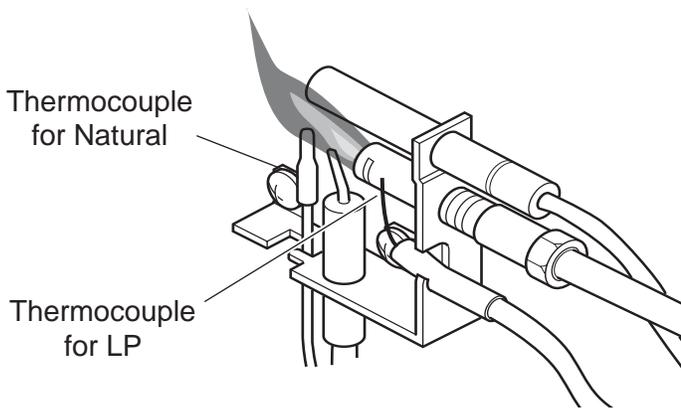
**Figure 30 - Correct Appearance of Pilot Flame**
