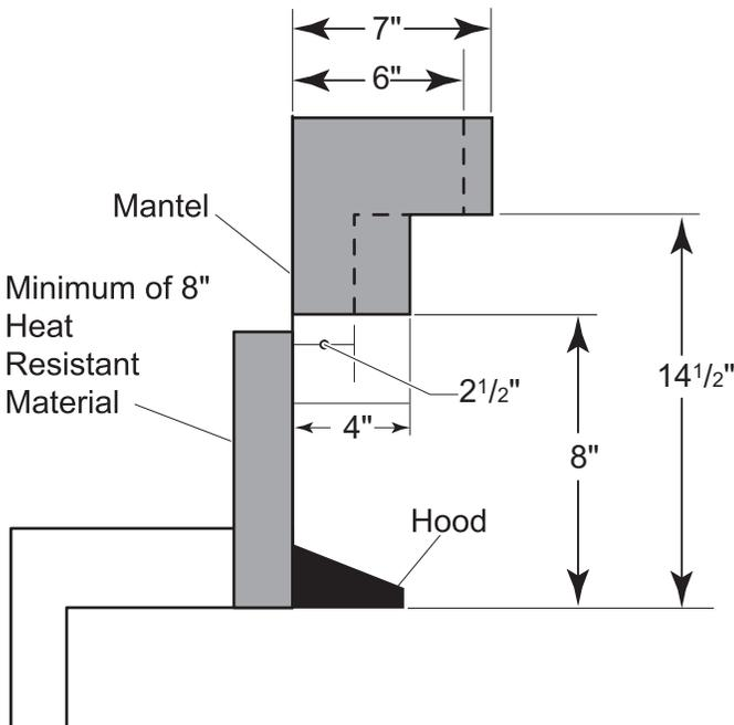
**Figure 10 is an example of an unsafe mantel installation.** This mantel projects 4" at 8" above the opening, exceeding the maximum acceptable distance of 2<sup>1</sup>/<sub>2</sub>". The mantel also projects 7" at 14<sup>1</sup>/<sub>2</sub>" above the opening, exceeding the maximum acceptable distance of 6".
