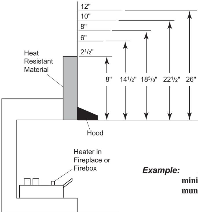
**Example:** A mantel may project from the wall a **maximum** of 2<sup>1</sup>/<sub>2</sub>" at a **minimum** of 8" above the opening, and a maximum of 6" at a **minimum** of 14<sup>1</sup>/<sub>2</sub>" above the opening.
