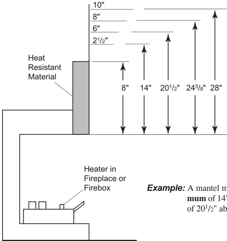
**Example:** A mantel may project from the wall a **maximum** of 2<sup>1</sup>/<sub>2</sub>" at a **minimum** of 14" above the opening, and a maximum of 6" at a **minimum** of 20<sup>1</sup>/<sub>2</sub>" above the opening.
