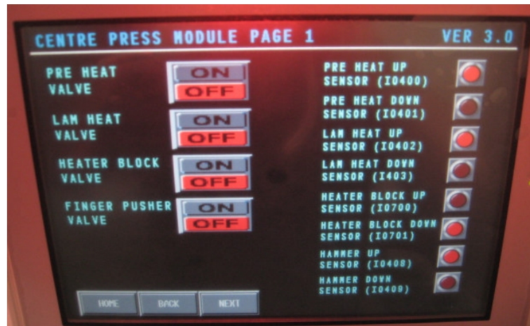
Figure 6-11: Maintenance Mode -Center Press Module Page 1 screen.
