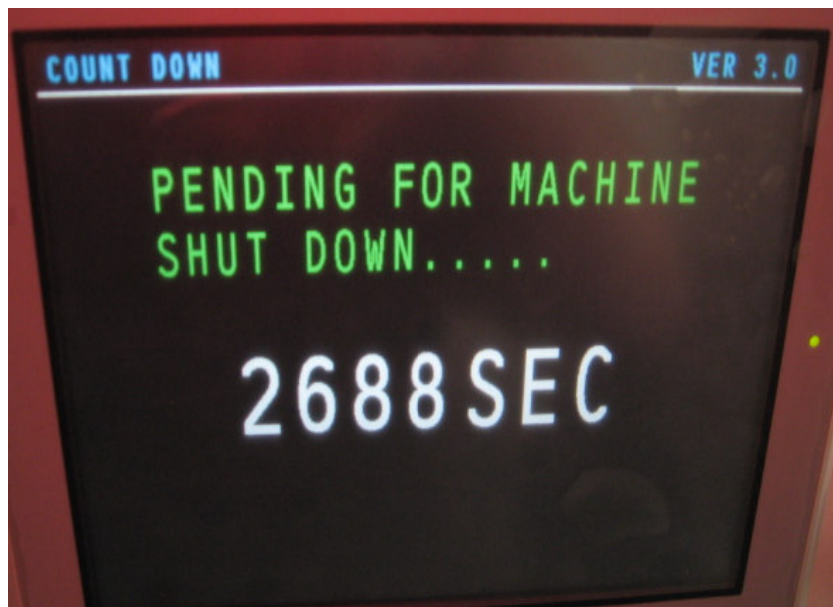
Figure 6-6: Maintenance Mode –Machine Shut Down Count Down Screen
