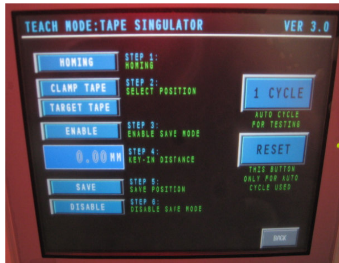
Figure 7-6: Teach Mode: Tape Singulator screen.
