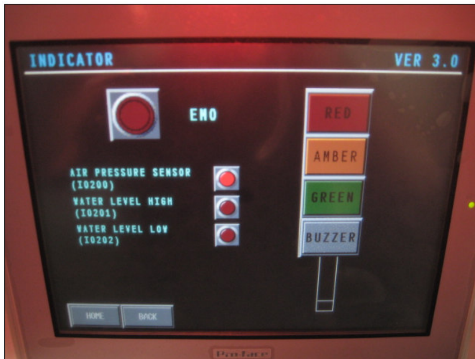
Figure 6-2: Maintenance Mode - Indicator screen.
