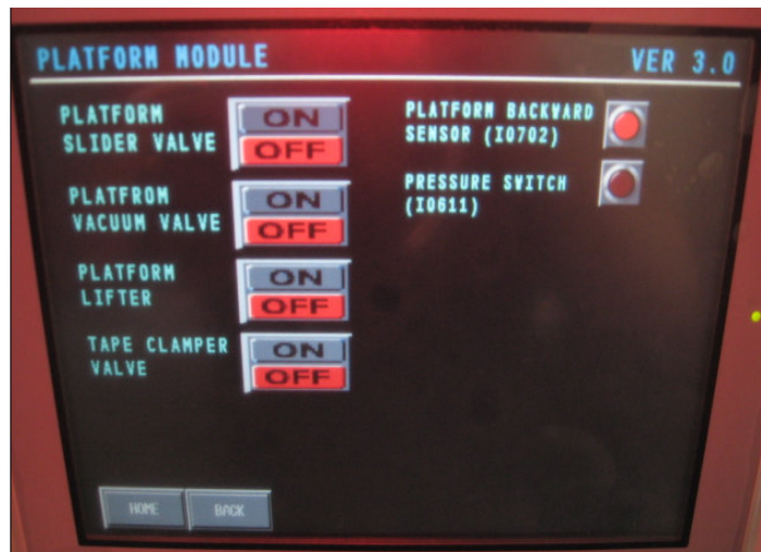
Figure 6-13: Maintenance Mode - Platform Module screen.
