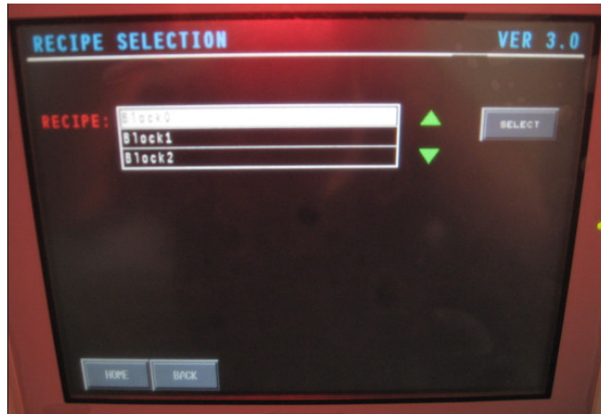
Figure 6-14: Maintenance Mode – Recipe Selection Screen.
