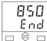
When the Timer ends, the Setpoint display shows alternatively the message  $\langle End \rangle$  and the Setpoint value until a key is pressed.
