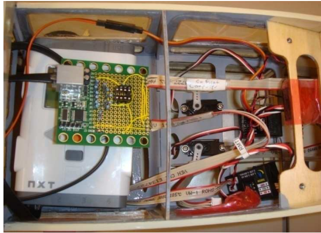
Figure 29. Hardware installation inside the aircraft model (Taylorcraft450)
