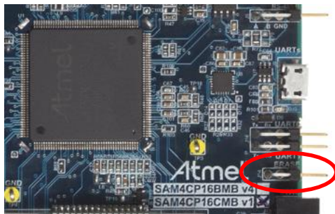
Figure 3-7. J14 jumper, ERASE.
