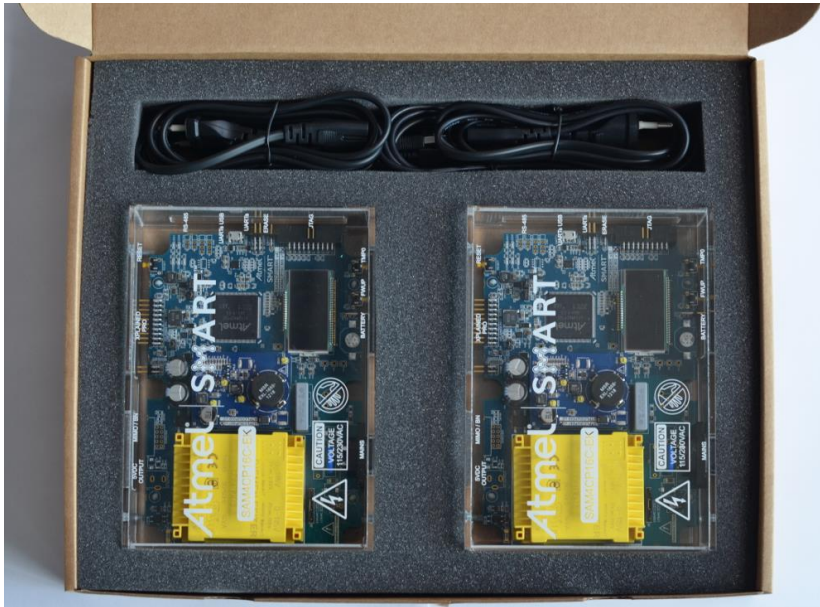
Figure 2-3. SAM4CP16CMB and ATPLCOUP007 boards.
