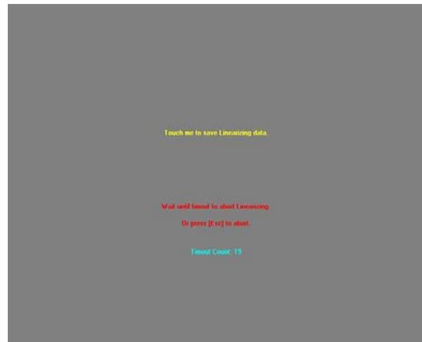
r. Touch any spot on the screen for saving linearizing data.
