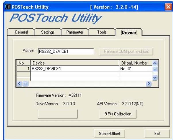
p. Select “Device” on the POS Touch Utility window, then click “9 PIs Calibration” button on the POS Touch Utility window.
