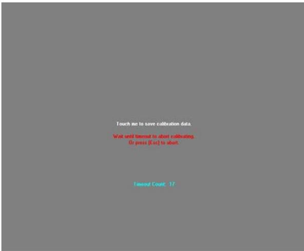
o. Touch any spot on the screen for saving calibration data.
