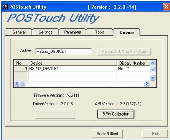
s. Click “Exit” button on the POS Touch Utility window, then the driver is installed now.
