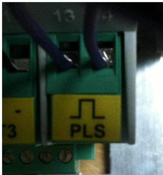
Note : Only use VOLT FREE pulse connections. Any other connections may cause damage to the Meter Logger and will void the product warranty. Crucible Technologies recommends using twisted pair wiring.
