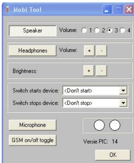
**Speaker Volume** button turns on or off the speakers. The number sets the gain of the internal audio power amplifier to a specific maximum. The recommended volume is 3. With a gain of 4, some distortion might occur depending on the nature of the audio that is amplified.
