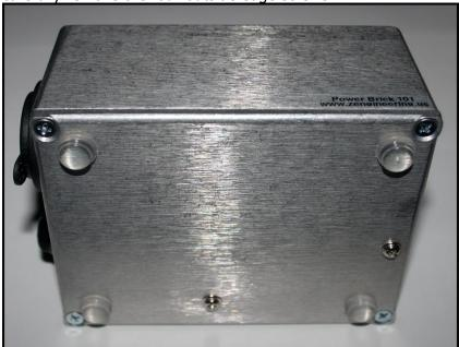
Gently lift the rear plate up and away from the Cigarette Socket end of the POWER BRICK™ as shown below.
