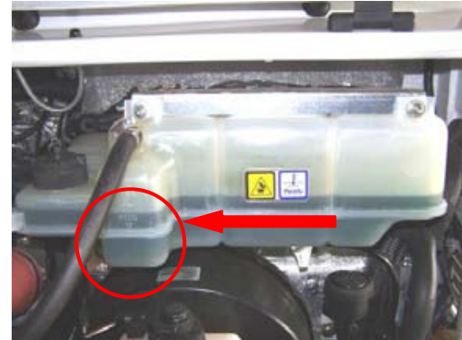
Cooling liquid tank
