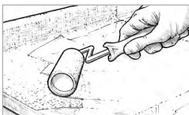
Figure 29 Coat the surface to fill the weave before the wet-out becomes tack free.
