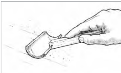
Figure 31 Tip off the coating by dragging a foam roller brush lightly over the fresh epoxy.
