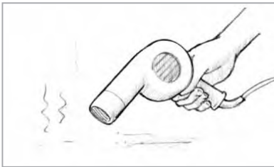
Figure 7 Dry the surface. Allow wet surfaces to dry thoroughly or use heat or a fan to speed drying.
