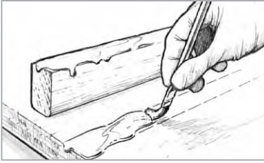
Figure 9 Apply resin/hardener mixture to the bonding surfaces.
