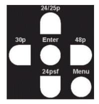
Press the **Menu** button to turn the OSD menu on or off. The highlighted (green text) cursor position in the OSD menu is maintained when the menu is turned on or off, so it is easy to turn the menu off when making measurements or adjusting a calibration setting, and then turn it back on again to make additional changes to the same menu item.
