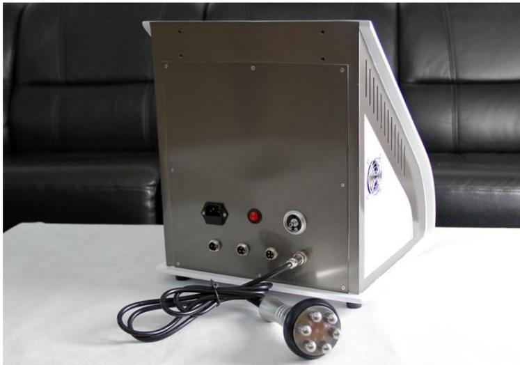
4. Connect the Body RF handle cable to the fourth connector.
