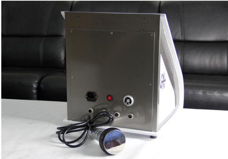
1. Connect the 40Khz Ultrasonic handle cable to the second connector.
