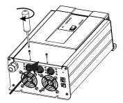
When all connections are made and double checked slide the red connection compartment cover to it's original position again and relocate the two screws.
