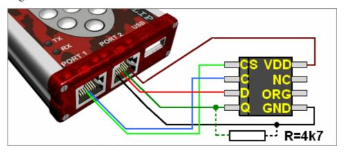
Some of chips needs to pull up GND to Q line via resistor. Resistance should from 2k to 10k. We suggest 4k7.
