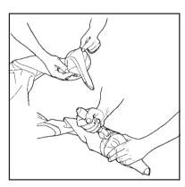
When using tape, apply two coats of glue to the area it will cover, on the outside.
