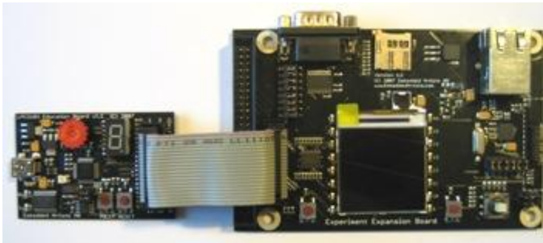
Figure 1 - LPC2103 Education Board with Experiment Expansion Board
