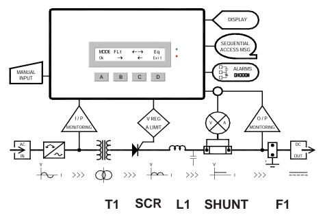
T1 — The AC supply is transformed and isolated.
