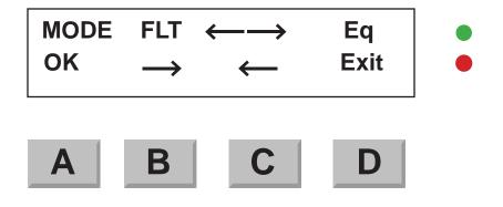
Press A (OK), to access the Float / Equalize menu. Press D (Exit) to step back to the menu screen.
