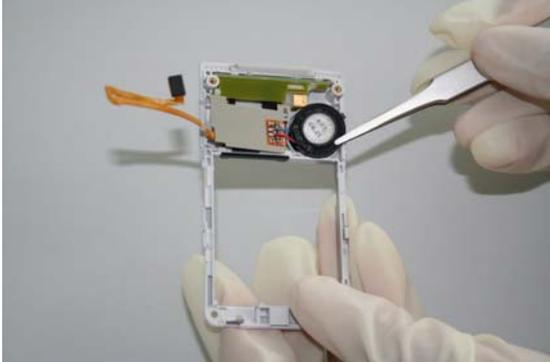
Assemble the Ringer-Alert by using Tweezers.
