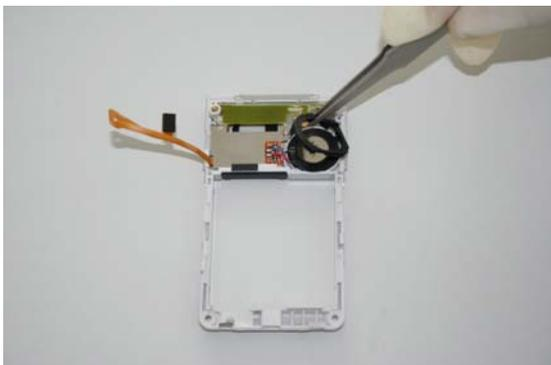
Assemble rubber gasket.
