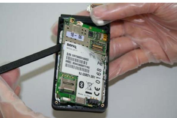
Remove the Keypad PCB.
