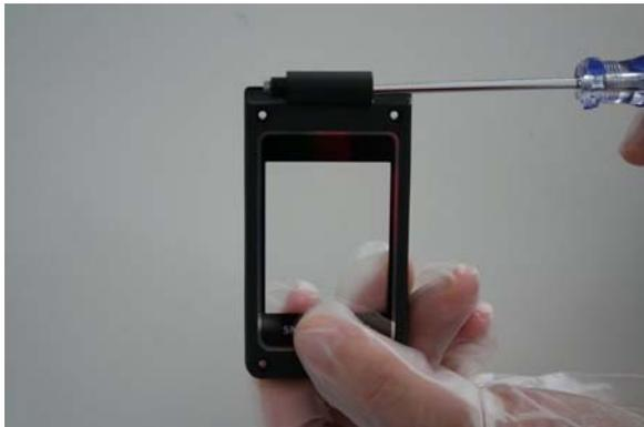
Remove the Ringer by using Tweezers carefully.
