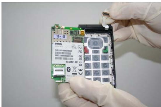
Assemble Keypad PCB.
