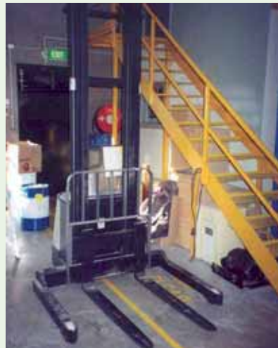
Electric walking stacker for moving bulk raw materials
