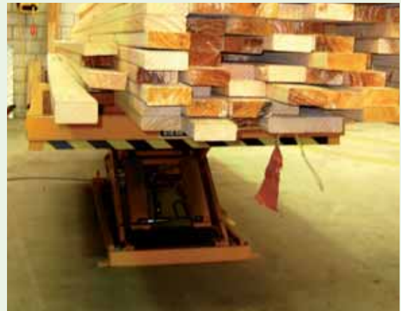
A spring lifter with a pallet ring in the photo above minimises reaching and forward bending for the employee
