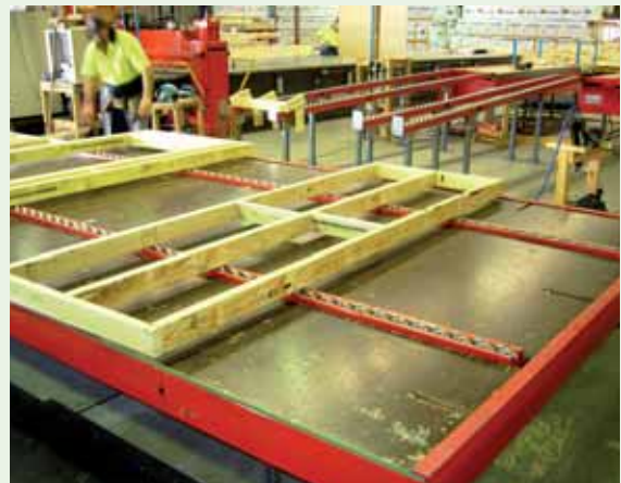
Retractable rollers on workbench to remove manufactured products
