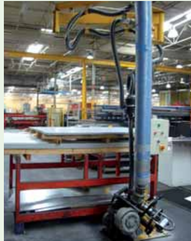
A vacuum lifter attached to a mobile jib crane
