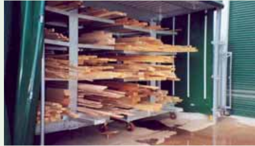
Mobile storage racking for raw material
