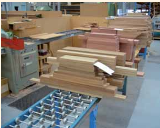
Fixed roller conveyors used to transport timber between work stations
