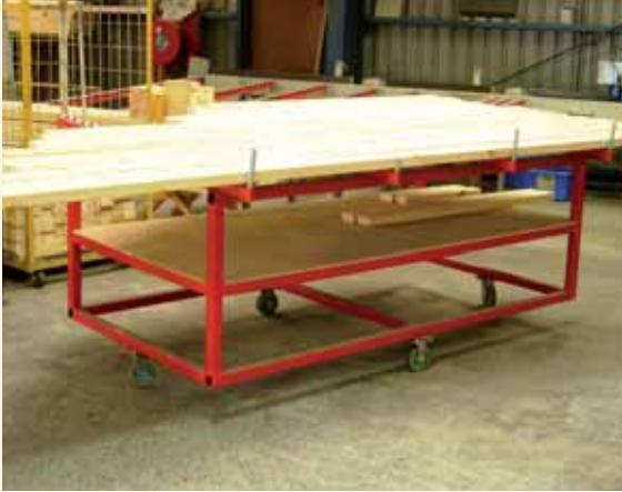
Trolley used to move cut lengths of timber to designated production areas.
