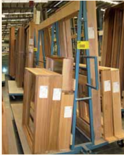
A-frame trolley used to transport window frames
