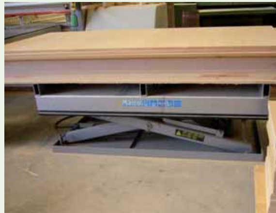
Scissor lift to raise boards of MDF to the correct height for transfer to wood working machinery
