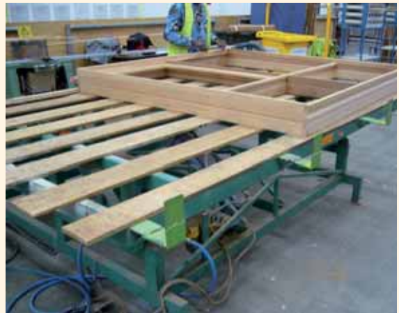
Tilt bench to transfer frame from work bench to trolley
