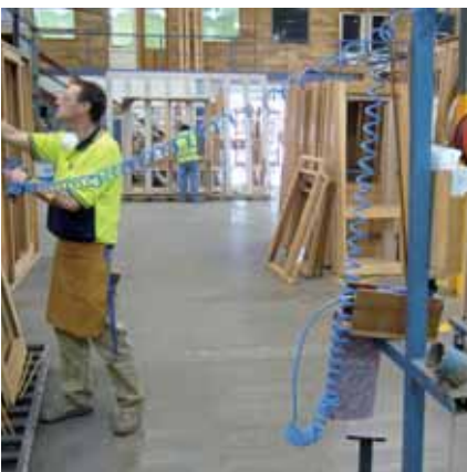
Stand with coiled air hose used to reduce clutter
