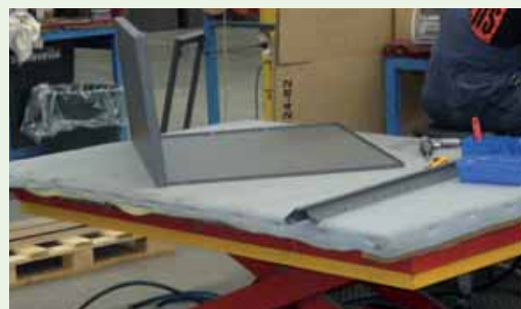
Hydraulic pallet lift table used as a work bench
