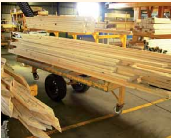
Trolley used for moving lengths of timber to production line
