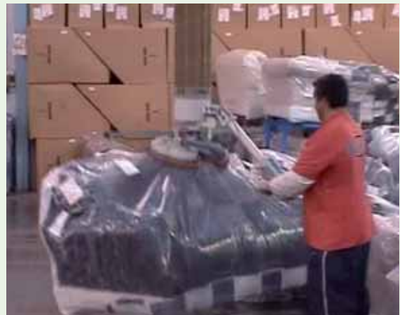
Vacuum lift is used to load sofas into stillages
