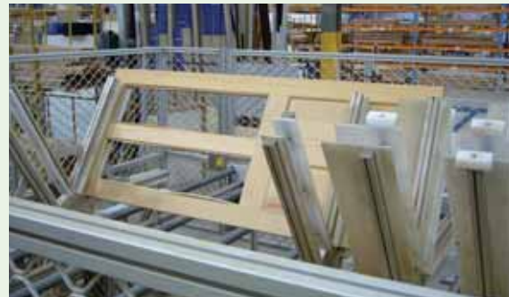
Inverter that automatically rotates a door on a sanding line.
