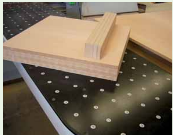
Air table uses compressed air and rollers to float the item so it requires a small force to move heavy timber along it
