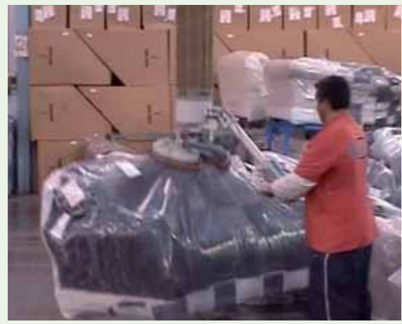
Vacuum lifter is used to load sofas into stillages
