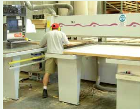
Handling heavy timber panels is made easier using an air table, as in the photo above.
