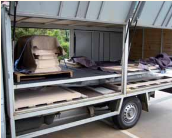
Specially designed trucks to load product at waist height
