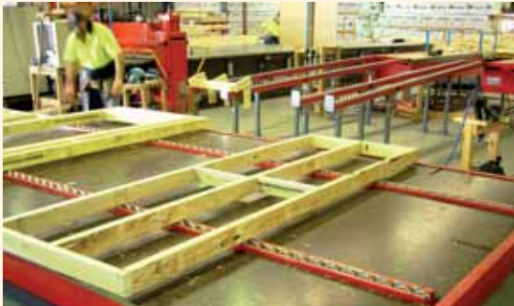
Rollers on work stations to move finished frames to stacks
