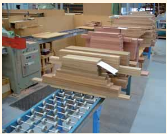
Extendable or moveable conveyors can be used to help move completed products
