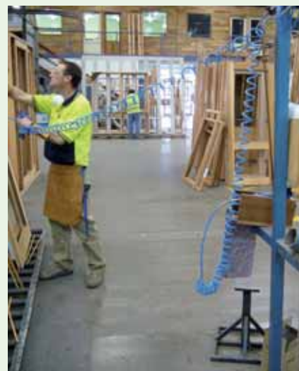
Stand with coiled air hose used to reduce clutter
