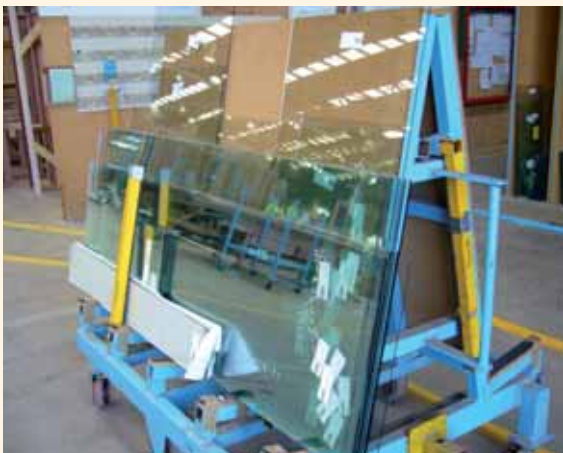
A-frame trolley used to transport glass
