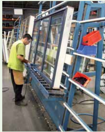
Height adjustable jig that forms part of a roller conveyor.
