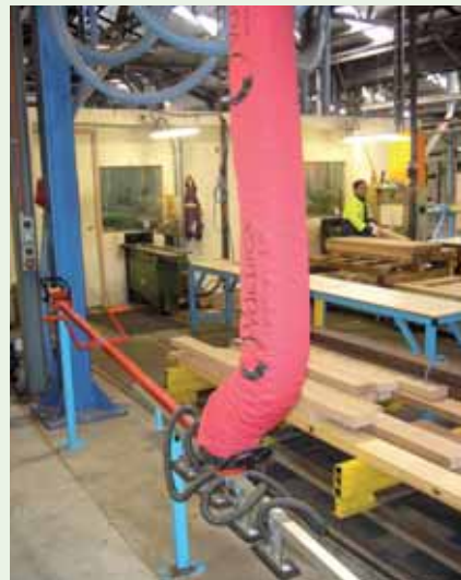
Vacuum lifter used to transfer raw timber to machine table
