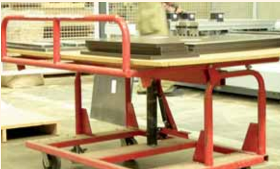
The trolley above is used to raise and orient the product for the employee
