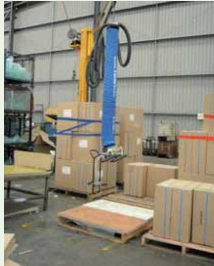
Vacuum lift is used to palletise finished product
