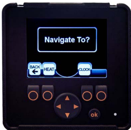
Clock Programming with Auxiliary Heater
