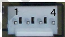
Figure 31: Onboard SATA Power Connectors
