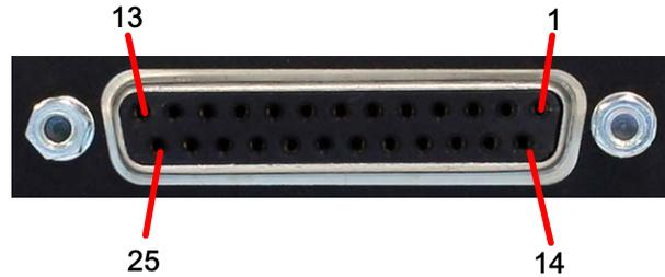
Figure 10: GPIO Connector
