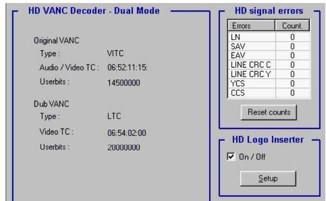
and the Dub VANC data. This data will be keyed as characters in the HD channel, and keyed as VITC+Characters into the SDI and Analog channels (PAL or NTSC) out of the downconverter (see VITC insertion below).
