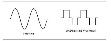
This modified sine wave has a root mean square (RMS) voltage of 115 volts. Most ordinary AC voltmeters are calibrated to read "average" voltage and assume that the AC waveform will be a pure sine wave. These meters will not correctly read MSW voltage, and will display about 20 to 30 volts too low. Any multi-meter identified as "TRUE RMS" will accurately read MSW correctly.
