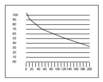
Continuing with the example above: The 150 amp load will need to run for 10 hours, so we begin configuration with a 1,500 AH battery. If the vertical is 1500 and the horizontal is 150 amps the percentage of load on the battery is 10 percent. The curve shows that the 1500 AH is derated to 90 percent of maximum. This means that the battery will have to be 1,650 AH for the full 10 hour run time. It is important to add some extra battery capacity, to compensate for battery age.
