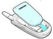
6. Press the battery until it clicks into place. Make sure that the battery is properly installed before switching the phone on.
