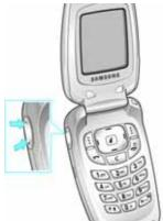
In Idle mode, you can also adjust the keypad tone volume using these keys.
