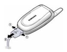
**Note:** You must unplug the adapter before you remove the battery from the phone during charging; otherwise, the phone could be damaged.
