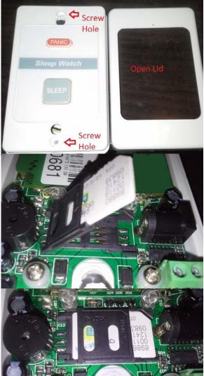
Remove lid and remove two screws to be able to open back housing.
