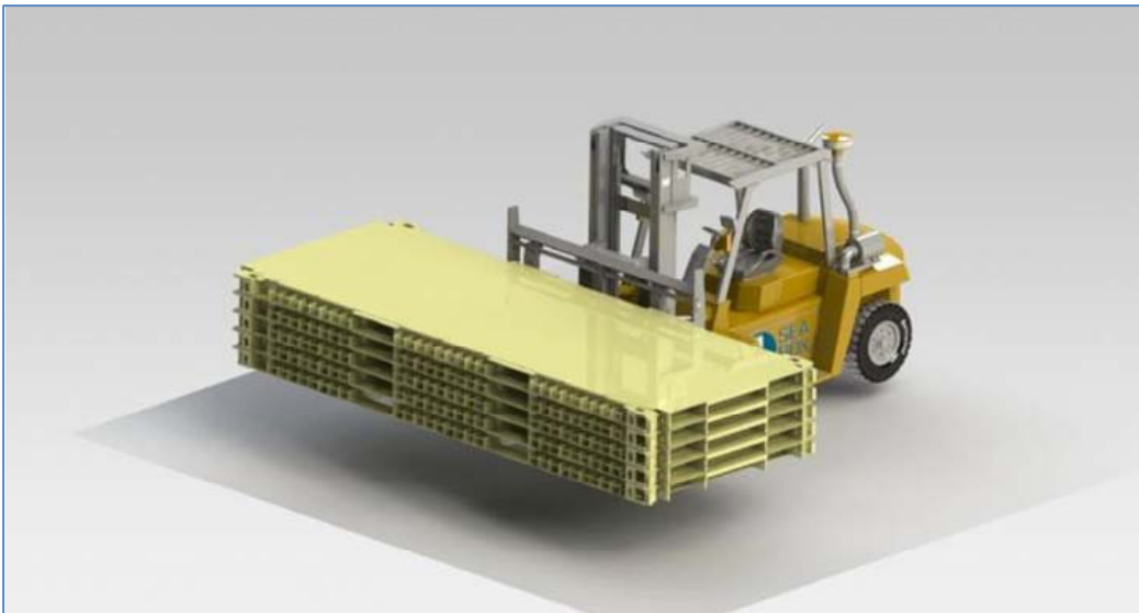
Figure 26: Lifting Nested CROWS from Side Fork Lift Pockets
