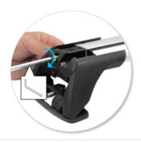
Tighten adjusting screw to 5 Nm.
